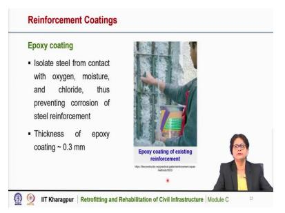
Epoxy coating actually isolate the steel from the contact of oxygen, moisture or chloride, thus preventing the corrosion of steel reinforcement the thickness is also much less in the order of 0.3 millimeter, here is one picture of epoxy coating of existing reinforcement, we can see that the reinforcements are exposed and the epoxy coating is applied on the exposed reinforcement to prevent corrosion.
