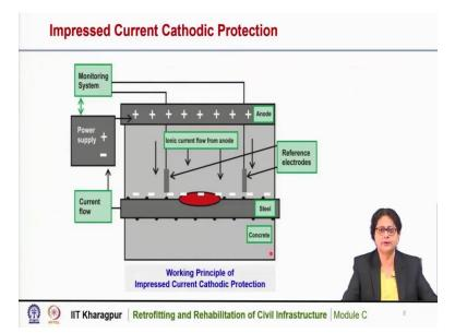
This is the working principle of impressed current cathodic protection. You can see here this is the existing concrete structure and this is the steel reinforcement, this part is the portion which is affected due to corrosion. Now, power supply is attached to the external anode and that is connected to this external anode and the reinforcement. There are 2 reference electrodes.
