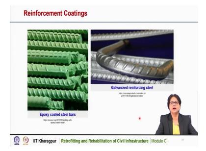
These are the pictures of reinforcement coating, one is with epoxy coating, these are the pictures of epoxy coated steel bar and this is a picture of galvanized reinforcing steel. So, these are effective measures and that can be taken for the protection of steel reinforcement against corrosion.
