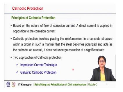
The cathodic protection principle is based on the nature of flow of corrosion current. Here in this technique a direct current is applied in opposition to the corrosion current. Corrosion treatment is done in this cathodic protection that involves placing the reinforcement in a concrete structure within a circuit in such a manner that the steel becomes polarized and acts as a cathode. As a result, it does not undergo corrosion at a significant rate.
