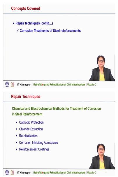
Today, we will continue the repair techniques; we will discuss several corrosion treatments of steel reinforcement in existing structures. There are several chemical and electrochemical methods for treatment of corrosion of steel reinforcement. We will discuss the cathodic protection, chloride extraction technique, realkalization and also we will discuss the corrosion inhibiting admixtures and reinforcement coatings which are used to treat the corrosion in reinforcement.
