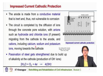
The anode is made from a conductive material in case of impressed current cathodic protection and the conductive material is inert and thus is not vulnerable to corrosion. The circuit is completed by the diffusion of ions through the concrete pore solution with anions such as hydroxide or chloride ions migrating from the cathode to the anode and cations including the calcium sodium or potassium ions moving towards the cathode.
