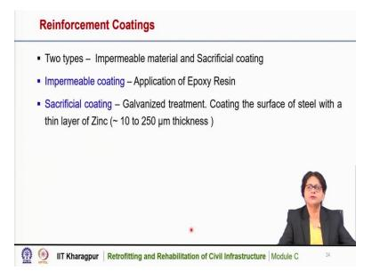
In case of reinforcement coating, there are two types of reinforcement coating that are used. One is by impermeable material and one is by the sacrificial coating. Impermeable coating is by the application of epoxy resin and in sacrificial coating it is the galvanized treatment. The coating of the surface of steel with a thin layer of zinc and the thickness is in the range of 10 to 250 micron.
