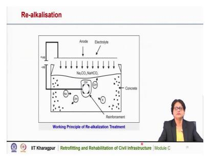
So, this is the schematic diagram of the working principle of re-alkalization treatment. We can see that this is the concrete and this is the reinforcement and this is the external anode which is placed on the surface. Two are connected with the power supply, the electrolyte used maybe sodium carbonate or sodium bicarbonate.
