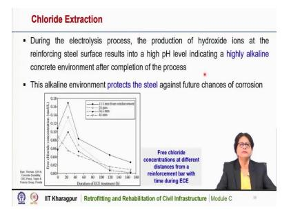
During the electrolysis process, the production of hydroxide ions at the reinforcing steel surface result into a high pH level, indicating a highly alkaline concrete behavior after completion of the process. So, OH ions are formed because that is the cathodic region, OH ions are formed and that results into the high pH level or the high alkalinity in that region. This alkaline environment protects the steel against further chances of corrosion.
