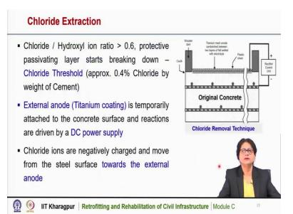
Chloride or hydroxide ion ratio when it is more than 0.6, the productive passivating layer starts breaking down. So, there is a chloride threshold which is approximately 0.4 percent of chloride by weight of cement and due to the chloride induced corrosion when the chloride by hydroxide ion ratio exceeds 0.6, then the passivating layer starts breaking.
