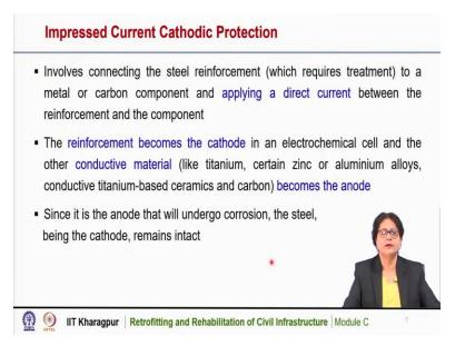
In impressed current cathodic protection, the method involves connecting the steel reinforcement to a metal or carbon component and we apply the direct current between the reinforcement and the component. So, the reinforcement becomes the cathode in the electrochemical cell and the other conductive material behaves as an anode.
