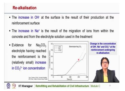
So, the increase in the OH ions at the surface is the result of their production at the reinforcement surface. The reinforcement now behaves as a cathode and so, there is the OH ion formation and that is produced and it is migrating to the surface. The increase in the OH at the surface is due to the production of the OH ions and the reinforcement.
