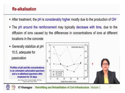
After the treatment the pH is considerably higher mostly due to the production of OH- ions at the reinforcement region or at the catalytic region, the pH around the reinforcement may typically decrease with time due to the diffusion of ions caused by the differences in concentration of ions at different locations in the concrete.
