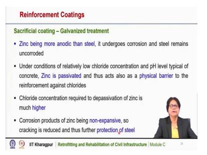
In case of sacrificial coating, it is the galvanized treatment that is being done and zinc is used for that purpose. Zinc being more anodic than steel, so it undergoes corrosion and steel remains and
