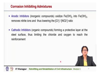
Anodic inhibitors are generally inorganic compounds, they oxidize a  $Fe(OH)_2$ , or ferrous hydroxide into ferric hydroxide and removes the nitrite ions. Thus, the there is a lowering of the chloride to nitrite ratio. So, this is advantageous because it increases the chloride threshold level.
