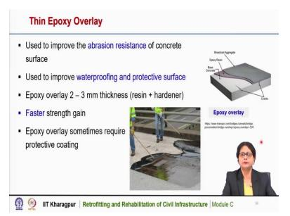
Overlay can also be by thin epoxy layers. So, this type of overlay is used to improve the abrasion resistance of the existing concrete surface and also to improve the waterproofing characteristics and to protect the existing surface. So, this is a typical picture of epoxy layer which is placed on the existing surface as an overlay, the thickness is much less in case of epoxy overlay as compared to the polymer overlay, it is in the range of 2 to 3 millimeter.
