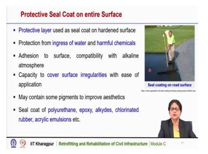
Protective seal coat on entire surface. So, here this also can be used on road surfaces which are maybe irregular and have surface irregularities. So, this type of protective seal coat is used on existing surface, particularly to seal the surface from the ingress of water and other harmful chemicals.
