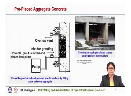
So, here is also a one schematic diagram shown this is also a wall type of structure and this portion is damaged. So, here formwork is made and the graded aggregates need to be placed, the, the grouting material, the cements and grout needs to be pushed into it inserted through force and then it is to be filled up and when the excess grouting material is coming out through this overflow vent then we can understand that the grouting is completed. So, then we can stop it.
