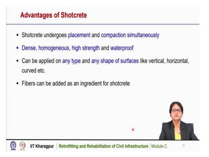
The advantages of shotcrete are several. That shotcrete undergoes placement and compaction simultaneously. We do not require any formwork or any other vibrator for the concrete to be applied. So, it undergoes placement and compaction simultaneously. We get a dense homogeneous, high strength and waterproof material through shotcreting. So, that is why it is
