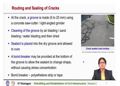
In routing and sealing, the groove is made at the crack phase using a concrete saw-cutter or rightangled grinder. So, we can use a simple saw-cutter or a grinder to have a groove at the face of the crack. And then the groove needs to be cleaned by your blasting or sandblasting or water blasting and it is to be dried up. After drying up the crack we need to place the sealant into the groove and then it is allowed to dry or cure.
