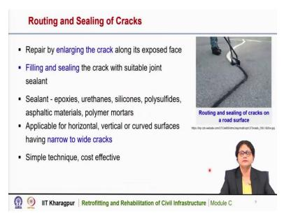
Routing and sealing of cracks are another type of crack repair method this is quite common, particularly when the crack is long and on a large structure like a slab or road surface, we can use routing and ceiling type of technique for crack repairing. The method involves enlarging the crack along its exposed face, then the crack face is filled up and sealed with some suitable sealants.
