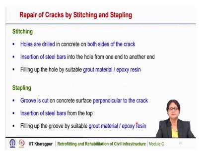
Stitching and stapling are another types of crack repairing and it is widely used particularly for structures which are damaged due to several cracks on it. In stitching holes are drilled on the concrete surface on both sides of a crack. If a crack is quite long, then we have to drill holes on both sides of the crack and that hole should go beyond the crack. Then in that hole, we have to insert steel bars from one end to another end.
