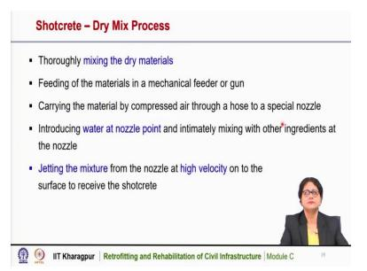
In dry mix process of shotcreting the materials are mixed in dry, that means all the ingredients they are mixed in the feeder in dry condition and then it is feeded into the mechanical feeder or gun. Now the dry mix is carried into the equipment and it is then carried by compressed air through a hose to a special nozzle.
