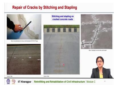
These are some of the pictures of stitching and stapling of concrete roads, here you can see this is the crack and this is the groove which is made for stapling purpose. Here is, this is the crack along the length of the road and these are the holes for stitching. So, after stitching the holes are filled up with epoxy resin and we can see here, alternating holes have been created on this both sides of the crack and steel bars are inserted and it is then filled up with grout or epoxy.
