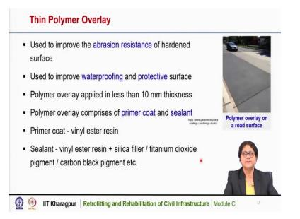
Sometimes we can also use overlay to repair the cracks. Thin polymer overlay is used to improve the abrasion resistance of hardened surface. The overlay is also used to improve the waterproofing and also to protect the existing surface, the polymer overlays applied in less than 10-millimeter thickness and it comprises of a primer coat and a sealant.
