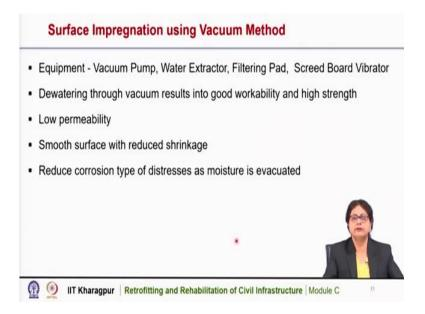
The equipment required for surface impregnation is vacuum pump, water extractor, filtering pad, screed board vibrator, etcetera. Dewatering through vacuum results into good workability and high strength. It results into low permeability of the structure, the smooth surface with reduced shrinkage and reduce the corrosion type of distresses as moisture is evacuated.
