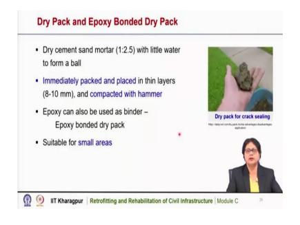
Now, there are several methods of crack repair, we can use dry pack, or epoxy bonded dry pack, for crack repair. Dry pack is a dry cements and mortar, generally, 1 is to 2.5 is the ratio of cements and mortar with little water in it, and that is why it is called dry pack.
