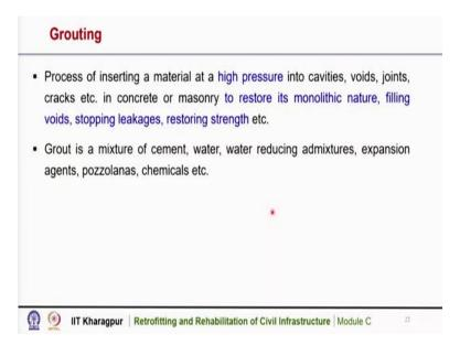
Grouting is a method used for crack repairing. It is a process of inserting a material at a high pressure into the cavities, or cracks, voids, joints, etcetera, on concrete surface, or masonry surface to restore its monolithic nature, to fill up the voids, to stop the leakages, and to restore the strength of the member.
