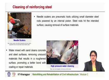
So, the cleaning of reinforcement steel can be done by needle scalers, or high-pressure water cleaning, as we have just mentioned. So, this is a picture of a typical needle scalers, needle scalers are pneumatic tools, which are utilized for the cleaning of reinforcement bars. And they have small diameter steel rods powered by an internal piston.
