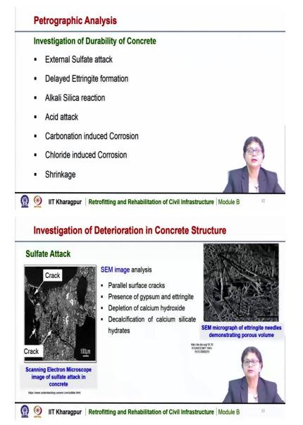
Petrographic analysis is quite effective for the existing structure's evaluation. We can investigate the durability of the structure. Various deterioration can be identified from the petrographic analysis. The external sulfate attack, the formation of delayed ettringite, the alkali silica reaction, the acid attack, carbonation etcetera can be found out from petrographic analysis.
