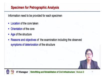
Specimens for petrographic analysis, generally we require very thin specimen, very small specimen because we need to test it under the microscope. So, specimen size is very small, but we also need some more information about the specimen. When the core is taken from an existing structure, we need to know the location of the core from where the core has been taken from the structure.
