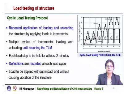
In case of cyclic load testing protocol, the load is applied repeatedly. It is the repeated application of loading and unloading of the structure by applying loads in increment. So, here also the load is applied repeatedly, but for each cycle the load is applied incrementally. So, here we can see that, at each cycle, the load is applied incrementally and multiple cycles of incremental loading and unloading is there until it reaches the TLM.
