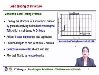
The monotonic load testing protocol is that the loading of the structure is to be done in a monotonic manner, by gradually applying the load until reaching the TLM, which is maintained
