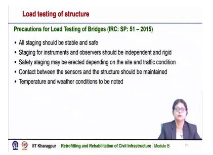
For load testing of bridges, we have to take care of several considerations, several precautions need to be taken. The precautions are all staging should be stable and safe. The staging because on the staging, people need to stand and carry out the test or are carrying out the measurements. So, the staging should be stable and safe. Staging for instruments and observers should be independent and rigid.
