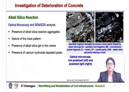
Alkali silica reaction can also be identified from petrographic examination, using optical microscopy and scanning electron microscope analysis. The presence of alkali silica reactive aggregates or the nature of crack pattern can be identified from these pictures and the presence of alkali silica gel in the cracks or presence of calcium hydroxide also can be found out from these microscopic studies.
