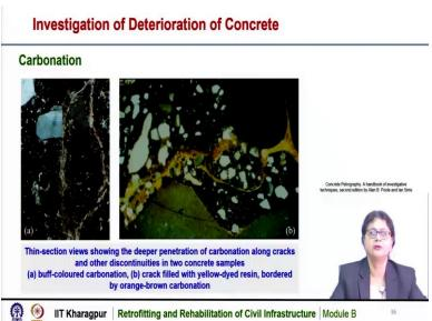
Carbonation type of distresses can also be identified from petrographic analysis. Here are some pictures. The thin section views showing the deeper penetration of carbonation along the cracks and other discontinuities in two concrete samples. We can see here there are two concrete samples and due to the effect of carbonation there are cracks developed along the material and the left side identifies the buff-coloured carbonation area.
