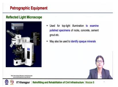
This is a picture of reflected light microscope. This is used for top light illumination to examine the polished specimens of rocks, concrete or cement grout etcetera. And this can also be used to identify different opaque materials. So, reflected light microscope is also another type of petrographic equipment, particularly used to examine the polished specimen.
