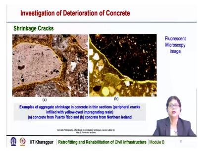
Shrinkage cracks can also be identified much clearly using several of the microscopes. Here are some pictures of fluorescent microscopic image and we can see here that the examples of aggregate shrinkage in concrete in thin sections, the peripheral cracks infilled with yellow dyed impregnating resin. So, here also while doing the test, the yellow-colored resin is impregnated, so, that the cracks are filled up with that and it can be identified easily.
