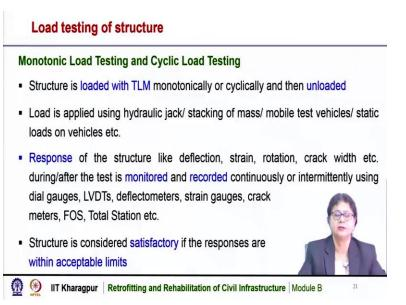
The load testing of structures can be done in two ways one is monotonic load testing and another is cyclic load testing. The structure is loaded with TLM either monotonically or cyclically when
