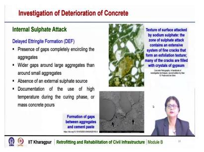
Internal sulfate attack can also be identified with a petrographic analysis. The delayed ettringite formation can be found out when we can examine the material. We can also find out the presence of gaps completely encircling the aggregates which is due to the delayed ettringite formation. There are gaps around large aggregates as compared to smaller aggregates.
