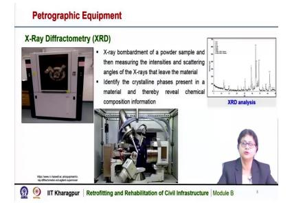
This is X-ray diffractometer or XRD. XRD, we can see here this is the XRD equipment and this is the inside of that equipment. And in this testing, it is X-ray bombardment of a powdered sample is done and then we can measure the intensities and scattering angles of the X-rays, that
