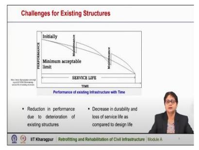
As a result, the service life of the existing infrastructures is reduced and they are facing the challenge of performance and durability. Look at this diagram, this is the performance with time variation of the existing infrastructure. When the infrastructure is constructed, the performance is maximum, but over a period of time the performance is reduced.
