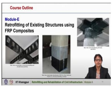
In Module E, we will cover the retrofitting measures of existing structures using FRP composites. So, here in this module, we will discuss, how we can retrofit an existing structural component using fiber reinforced polymer composites and what are the analysis and design methods for this retrofitting. So, in Module E, we will discuss the retrofitting measures of existing structures using FRP composites.
