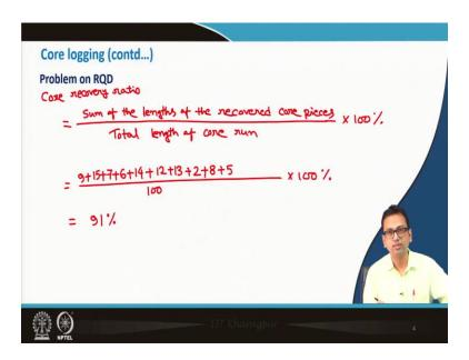
Core recovery ratio is nothing but the sum of the length of the recovered core pieces by the total length of core run. So, you know this is 100 centimeter.
