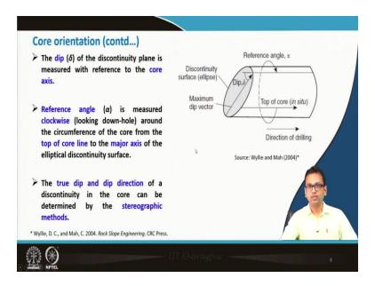
Next, we will discuss about another small topic, core orientation. What is core orientation? If the design data on discontinuity orientation are not sufficiently available from the surface mapping then it may required to obtain the orientation from the drill core. So, using the drill core you can get some useful informations regarding the core orientation. So, that is the idea which we will just discuss in brief.
