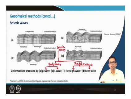
Now, seismic waves can be divided into two categories. First they are nothing but the body waves and surface waves. Now, body waves can be divided into two categories. They are P waves and S waves. Surface waves can be divided into 2 categories broadly. They are Rayleigh waves and Love waves. Again these waves can be divided into other two categories like S h wave, S v wave depending on horizontal and vertical orientation, means movements of particles. So, broadly these are the divisions.
