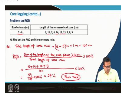
Regarding RQD and core recovery, we did a problem in our previous class. Another small problem, the data may be provided in this form (())(01:20). So, the problem is we need to find out the RQD and core recovery ratio. Here, the bore run is provided between 5 meters to 6 meters. And these are the lengths of the recovered bore core in centimeters. They are provided over here.
