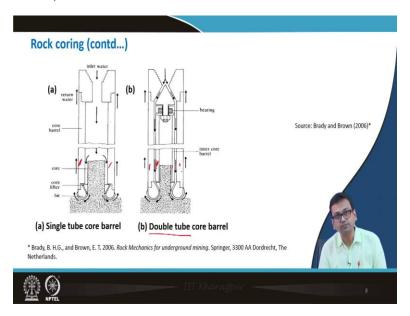
Let us see some pictorial representation of those things in Slide no. 8. The first one is single tube core barrel. So, there is only a single tube. This figure is representing the cross-section of the 3D diagram. The other one is the double tube. Here, two arrows are shown in double tube core barrel.
