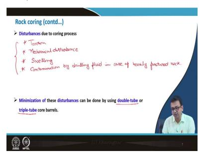
Based on past experience, we know that the disturbance due to coring process is quite common thing. So, the disturbance due to coring process can be due to
