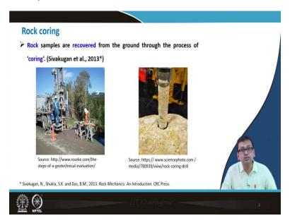
We will start with rock coring. Rock samples are recovered from the ground through the process of coring. So, how it is done? From slide, you can see big machineries are there, and you can see that the coring operation is going on. Cylindrical sampler is there which is inserted here. So rock samples are recovered from the ground through the process of coring.
