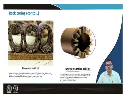
In slide no. 6, you can see the pictures of the diamond drill bit and tungsten carbide drill bit. It can be identified that the thickness is quite high for the both the types of drill bit. The front arrangement of tungsten carbide drill bit can be observed from the slide no. 6.
