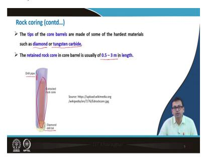
Here, we can see that the tips of the core barrels are made with some of the hardest materials. As it is known that diamond and tungsten carbide are very hard material, the tips of the core barrels
