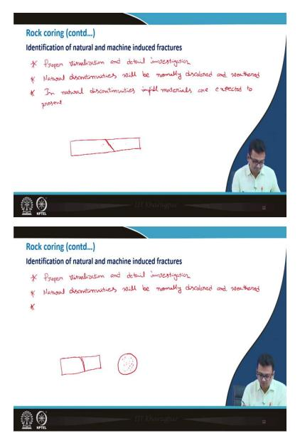
So, there are some ways of identifying the fracture whether it is manmade or natural. The basic idea is by proper inspection. This idea obviously will develop with experience in the field of rock mechanics. But some of the things what we can write regarding these are maybe the proper visualization and detail investigation.
