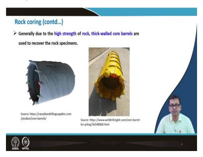
Now, from this diagram, you can understand, generally due to the high strength of a rock, thick walled core barrels are used to recover the core specimens. So, you can see from figure that it has a quite thick walled. The material with which it is made of, must be having high strength. So, we can say that generally due to the higher strength of rock, thick-walled core barrels are used to recover the rock specimens.
