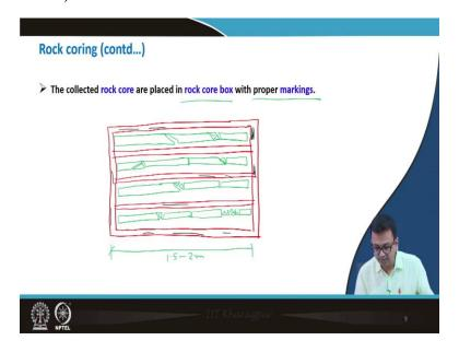
Another important thing is needed to be discussed. The collected rock cores are placed in the rock core box with proper markings. Markings in the rock core box are very important to identify the samples for future usages. The top view of a rock core box is drawn here in slide 9. It should be strong enough to keep the rock cores. In addition, there should be different compartments as
