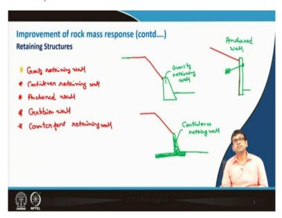
Then, retaining structure. So, we I am sure you know about different types of retaining structures, like retaining structures are like, you must be knowing about gravity retaining wall. Then, you must be knowing about this cantilever retaining wall, then you also know about anchored wall. Then, there maybe another type of wall, the Gabbian wall; or maybe counter fort retaining wall, means whatever.
