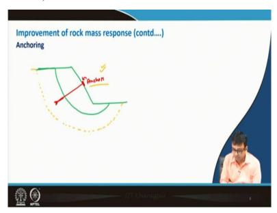
Now, other than that, what can be done by providing anchor; so, as we have learnt already. So, if your failure surface is like this; then, what may be done? We can, we can go for anchor; so can go for anchor; so, this is the anchor. Now, if happens like, if the failure surface goes like this; then this anchor will be of no use.
