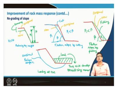
Let me just draw some of the things, what are the methods like one is reducing the height of the slope, one is flattening like flatter slope going for the fatter slope by filling or cutting or providing load. What I mean to say actually, let me try to draw two three diagrams for that. Suppose, initially this was the slope; so now what may happen?
