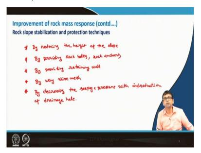
So, rock slopes stabilization and protection techniques. So, some what are mean how it can be done, let us write down some of the common techniques, like by reducing the height of the slope that can be one thing. And then maybe by providing rock bolts, rock anchors, rock bolts, rock anchors; then, also by providing retaining wall. Then, by providing steel like wire meshes, steel mats actually; so, by using wire mesh.
