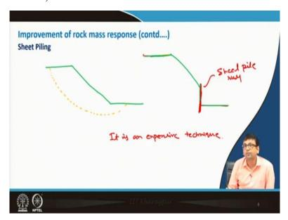
Like sheet piling is also I think one another type of retaining structure, but it is costly; so, anyway, let me draw the diagram. Suppose, what is happening, suppose this is the case. Now, it may happen that initially the failure surface is passing through this. Now, what maybe the way, then what maybe done is you can provide the sheet pile like this.
