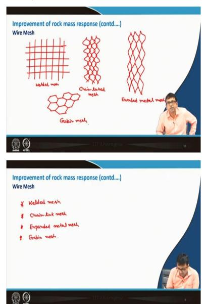
Welded mesh is simple like; it will be welded like this simple; these are the welded mesh, this is welded mesh. Now, in case of the second one that is the chain-link mesh; how it will look? It will be something like, likewise here also it will be like this; I hope you are understanding what must have seen this type of mesh. This is nothing but the chain linked.
