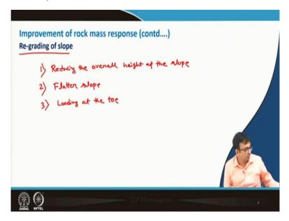
So first is re-grading of slope, means by reducing the height or some other techniques like what we can do. So, re-grading of heights under that that one thing maybe, as we have discussed that reducing the overall height that is fine. So, reducing the overall height of the slope, this maybe one thing; another thing maybe by cutting or filling the slope angle maybe reduced.
