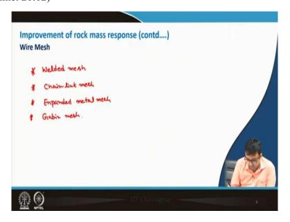
Now, wire mesh. Under wire mesh different type of wire mesh or steel mats can be provided. Let first is suppose welded, welded mesh; then, another type is chain-link mesh. Then, there is expanded metal mesh and here several types; so just I have written some of them like Gabin mesh. Let me just try to draw some of the diagrams like.
