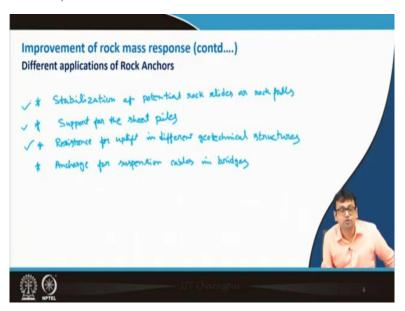
Now, different applications of rock anchors; so what are they? So some of the applications, it is used for stabilization of stabilization of potential rock slides or the rock falls. This can happen when for that purpose it is it can be used. Also support for the sheet piles that for that purposes it is use.
