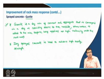
Now, a little more if we discuss about this dry mix, how it is. So, it can be stated that that this gunite. So g u n i t e, so gunite is a dry mix of cement and aggregate. That is actually what is done, means that is conveyed in general in dry form, or almost in dry form, till the nozzle of the pipe through which it will be sprayed. And there is little amount of water is added to moist the thing.
