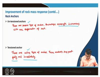
Now, these rock anchors are can be divided into two categories, like un-tensioned anchors and tensioned anchors. So now, what is this un-tensioned anchor? This basically these anchors are like passive type of anchors. These are passive type of anchor, and that is what we can say; and on the other hand, the this tensioned anchors are the active type anchor.
