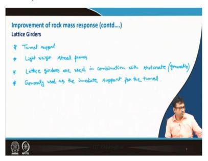
Now, another thing is lattice girders. So, lattice girder what is this? These lattice girders are, these are used for the, for constructing the tunnel supports. So, it is used for mainly for tunnel supports, for there it is used and these are very lightweight steel frames. Generally, these lattice girders are used with the along, this is used in combination with the shotcreting; we will learn about the shotcreting very soon.
