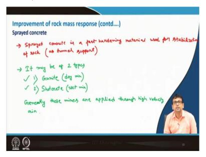
Now, sprayed concrete; so, this is again very important thing. Here only the shotcreting will again come. So, the sprayed concretes, these are the fast hardening material used for that purpose. And it is used mainly as for the for providing the support to the tunnel; when the tunnel excavation is going on. So, sprayed concrete is a fast hardening material, fast hardening material used for stabilization of rock, mainly as the, as or for simply that as tunnel support.
