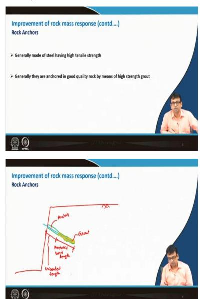
Rock anchors: So basically means, in general, these rock anchors are made up like this; mainly it is made of steel, and the steel should have high tensile strength. And generally they are anchored in good quality rock by means of high strength grout. So, this how it looks actually, just a simple schematic diagram if I want to draw.
