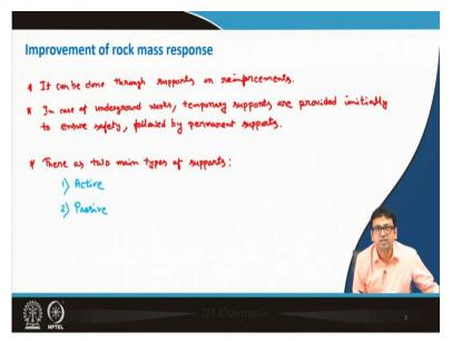
It can be done through may be by providing support, or by including reinforcement. So, first point may be written as, it can be done through supports or reinforcement; quite self-explanatory, means either suppose some slope is failing.
