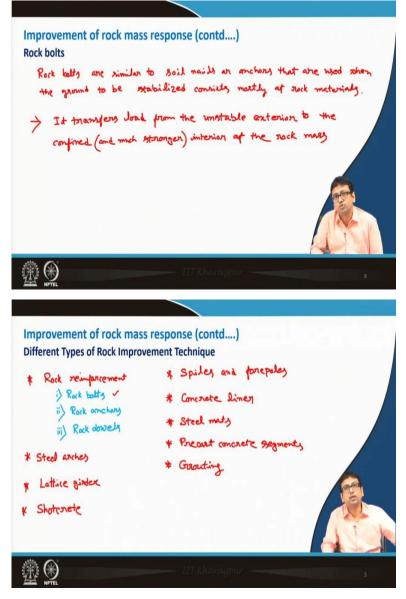
Now, rock bolts. So, rock bolts as I mentioned and written also over here; the first type of reinforcement is this rock bolt. What we will discuss first, so we will begin with the rock bolts today only. So, basically this rock bolting actually in soil, probably have heard about like soil nails and anchors.
