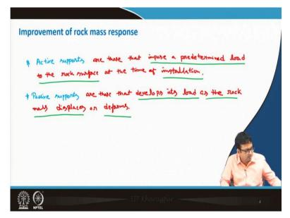
So, first is the active support. So, active supports are those that impose a predetermined load to the rock surface at the time of installation. On the other hand, passive supports are those that develop its load as the rock mass displaces or deforms. So, with deformation or displacement, it starts developing the load; so these are the basic differences, we should at least know what are they.
