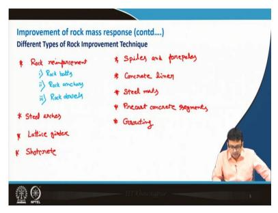
Now, different types of rock improvement techniques that is very important, which we will learn actually one by one in this module. So, some of the names we can write now, like first is of course the rock reinforcement. Now, under rock reinforcement, there maybe rock bolts like rock anchors, then rock dowels all these things are there; we will discuss about these things. So, rock bolts are used widely, in fact very widely used. Rock anchors, they are also very popular; and rock dowels.
