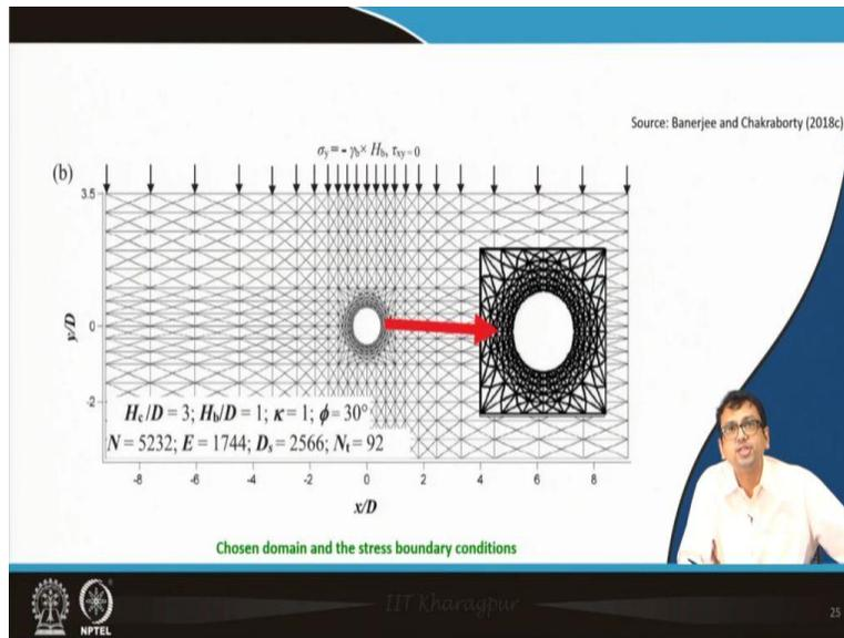
So, another work is the stability analysis of circular tunnel underneath fully liquefied soil layer. So, here also unlined tunnel has been considered and lower bound limit analysis is used. So, Banerjee and Chakraborty, this paper is published in Tunneling and Underground Space Technology.
