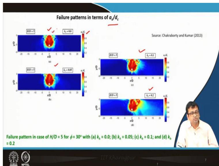
So, now we can see how the failure patterns look like. Now, here  $a_c/d_c$  is ratio that indicates plastic failure when it becomes one. Therefore, you can see deep red if it became 1. With  $k_H$  is 0, the failure pattern is very much symmetric.
