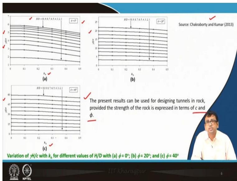
Now, the end product plots are given in the paper if you follow it; you Here only three plots are shown by phi value of 0-degree, 20-degrees, 40 degrees. It is the variation of  $\gamma H/c$  versus  $k_h$ .  $k_h$  is horizontal seismic coefficient; and  $\gamma H/c$  is nothing but the stability number.  $\gamma$  is the unit weight of the material, and  $H$  is the crown depth from the ground surface and  $c$  is nothing but the cohesion of the soil.
