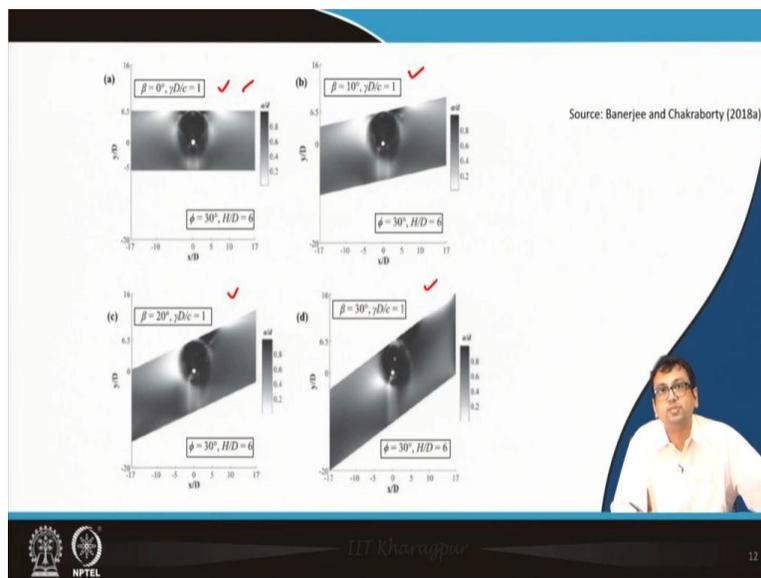
Now, stability of long circular tunnels in sloping grounds. This work is for a pressure tunnel. In our previous lecture only, we have discussed about pressure tunnel. So, a uniform pressure,  $P$  is applied; lower bound finite element limit analysis used for this problem also. Here also all the codes were written in MATLAB.
