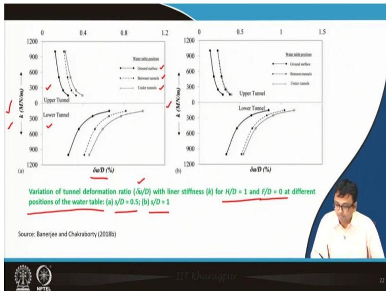
Then a representative plot for the variation of tunnel deformation ratio that you have present in terms of  $\delta u/D$ , with liner stiffness. Liner stiffness presented for  $H/D = 1$ ,  $F/D = 0$  at different positions of water table, for  $s/D = 0.5, 1$ . So, water table at ground surface, between tunnels, under tunnels is shown; and upper part of the plot is for upper tunnel, lower part is for lower tunnel.
