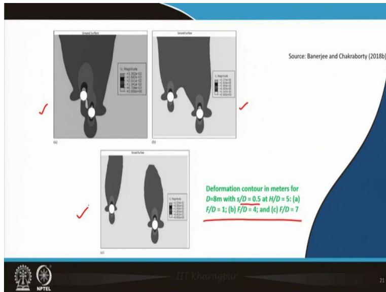
Now, for second set of results,  $s/D = 0.5$ ; and  $F/D = 1, 4, 7$ . For  $F/D = 1$ , the deformation contour is very much overlapping, for higher values the overlap reduced and for  $F/D=7$  it has completely separated from each other. So, that is one important observation.
