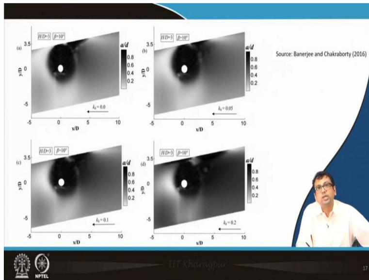
Again, there are some of that failure pattern, again the same thing  $a/d$  equal to 1 indicates failure.
