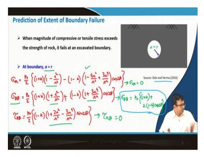
Suppose there is a tunnel, and at boundary a = r, no confusion. Now, when the magnitude of compressive or tensile stress exceeds the strength of rock, it fails in an excavated boundary. Now, we know
