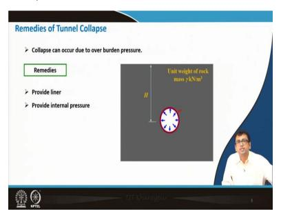
Collapse can occur due to overburden pressure. And you know different stresses are there, because of which it may fail. Remedies are to provide liner or provide internal pressure or both. So, these two are the simple solution what comes to our mind immediately. So, let us learn more about this these remedies.
