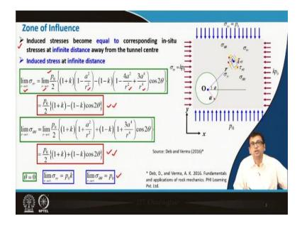
Now, just before starting the problem let us revise the last topic. So, in our last lecture we discussed about the zone of influence. I stated that the induced stresses become equal to corresponding in-situ stresses at infinite distance away from the tunnel center, which means at about an infinite distance, the effect of tunnel will not be there. That is why at that location it will be nothing but the in-situ stress.
