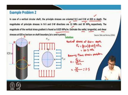
So, these are the tangential and radial stresses are at a and b both are equal to 0 and shear stresses at a and b both are equal to 0 and if you consider vertical stress which we have obtained here that is though it is not asked but just we have obtained it is 20.5 mega Pascal, so in this way we can design the vertical shafts also using this Kirsch situation.
