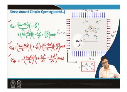
An Analytical formulation for a long circular tunnel in an ideal rock mass was developed by Kirsch (1898). The equation are expressed as
