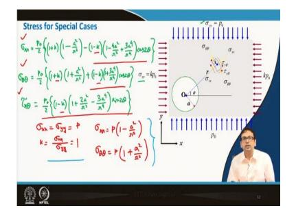
So, now another thing is a special case for like stress, for the special case, special case means what I mean to say here is suppose your  $\sigma_{xx}$  and  $\sigma_{yy}$  is equal, so then that means k will become equal to 1. So, now just let me just quickly write down the basic expression what we have written earlier also,
