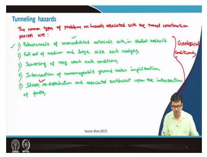
This book is a nice book that you can read for further details. Regarding tunneling hazards, there are the common types of these problems or hazards associated with tunnels construction. These tunnel construction processes are mostly related to the actual geological conditions. So, the main thing is geological condition other than that a few more sources are there. So, we will discuss about that one by one.
