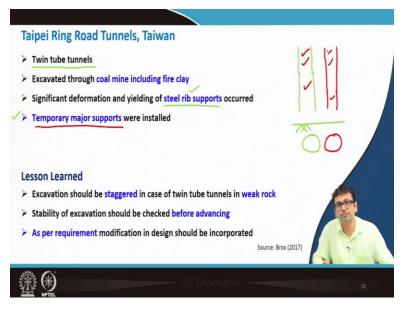
Now another one briefly I will discuss that is Taipei Ring Road Tunnel, Taiwan. So, here actually Twin Tube tunnels were constructed or Twin tunnels you can simply say and excavated through coal mine including fireclay. So, it was through a coal mine including this fireclay and apart from that, what other features are like significant deformation and yielding of steel ribs support occurred.
