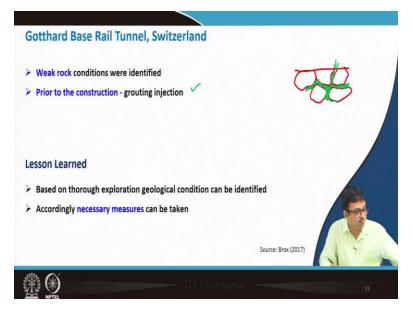
And now the last one I will discuss. The weak rock conditions were identified actually beforehand constructing the Gotthard Base Rail Tunnel, Switzerland. So, it is a rail tunnel. The good thing is before constructing only weak rock conditions were identified and based on the identification what was done prior to construction grouts were injected.
