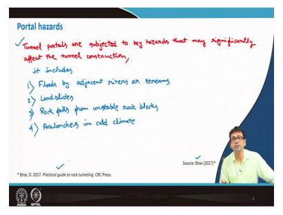
So, first one is Portal hazards as I mentioned. The tunnel portals are subjected to key hazards that may significantly affect the actually the tunnel construction.
