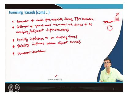
So, there may be some other few reasons also such as you see. So, generation of excess fine materials during this TBM excavation that may create one obviously hazard then obviously the another thing is you see because of constructing tunnel there may be the settlement of ground above the tunnel.
