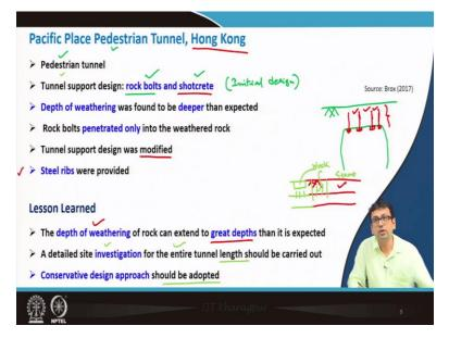
So, the first one is the specific place pedestrian tunnel in Hong Kong. So, as name suggests, it is a pedestrian tunnel. Now, initially it was decided that the tunnel the obviously before starting the construction process, so, we go for the tunnel support design. So, rock bolt and shotcrete was initially planned actually.
