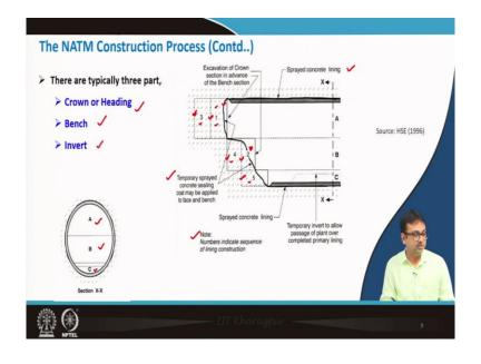
So, we can see that there are typically three parts as shown figure. One is crown or heading this part. Now, next is bench and third one is invert which is this part. So, these are the typical three parts. Now, you see the, this diagram is interesting you see here note that the like numbers 1, 2, 3, 4, 5 are given. Now, what is stated or written over here note numbers indicate sequence of lining construction.
