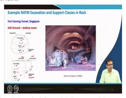
Similar type of figure is shown for Soft ground shallow cover and the process is only going on over here. You can see in the figure that the different zones is divided into that and like the top heading, bench, invert and here also 1, 2, 3, 4 here you see this is on the sectional view if you see
