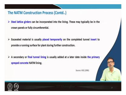
Now, this Steel lattice girders can be incorporated into the lining to give the ultimate or permanent lining. These may typically be in the crown panels or fully circumferential. The excavated material is usually placed temporarily on the completed tunnel invert to provide a running surface for plant during further construction.
