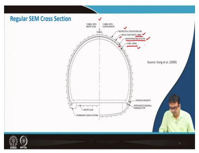
This is what regular SEM cross section. So, please look at this one very carefully, what are the components who can see it see it is the center line of the tunnel now, the layers you try to understand observe. So, this is as you can theoretical excavation line at initial shotcrete lining.
