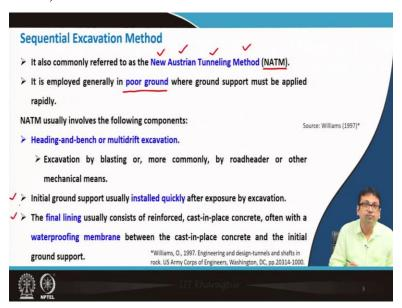
It also commonly referred to as the New Austrian Tunneling Method. So, New Austrian tunneling method in short is written as NATM. It is employed generally in poor ground where ground support must be applied rapidly. So, that is why I highlighted poor ground. This NATM usually involves the following components like heading and bench or multidrift excavation.
