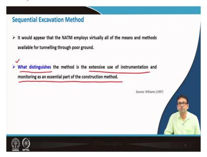
It would appear that in NATM employs virtually all the means and methods available for tunneling through poor ground. So, you can go for drilling and blasting or you can go for like road header. So, all these methods can be means are used in this in NATM actually. So, NATM means New Austrian Tunneling Method. So, which is also nothing but the sequential excavation method.
