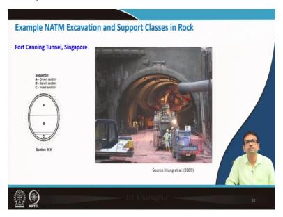
Now, you can see the Fort Canning Tunnel, Singapore. You can see that the tunnel was constructed is applying this SEM. So, you see that the excavation is going on. It will go proceed as I have mentioned in my previous slide, so, you can clearly visualize this part has been like excavated liners are putting
