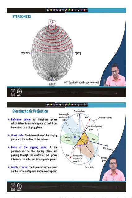
So, for that purpose, these stereonets are available in the market. Now what is this? As you can see, it is written over here 'A 2° Equatorial equal angle stereonet'. Now this is what? This is basically nothing but the horizontal plane what we have identified over here. And these curve lines are nothing but the great circles, you can imagine that is, all this line, so this line, you can consider as one great circle, this line, this line, likewise it is going.
