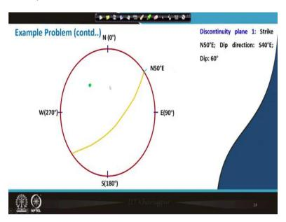
If I leave the tracing paper from the stereonet it will look like this. After identifying the discontinuity plane 1, which is having the strike as  $N50^{\circ}E$ , dip direction as  $S40^{\circ}E$  and the dip =  $60^{\circ}$  and the stereonet will look like this. So we will continue this problem in our next class. So,
