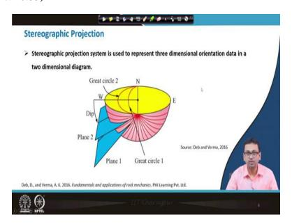
So, we have to understand, what is stereonet? How it is prepared and how it can be used for plotting the geological data on the stereonet. So, let us first understand the stereographic projection. Stereographic projection system is used to represent three dimensional orientation data in a two dimensional diagram. So if we can present the three dimensional orientation in a two dimensional diagram then our life becomes relatively easier.
