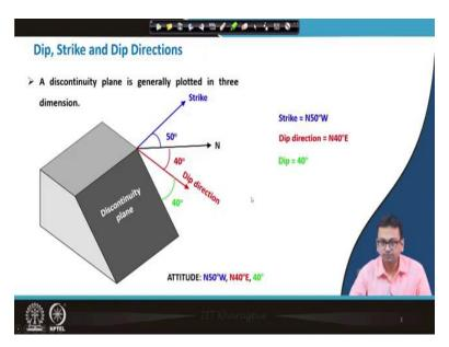
So, I have already told you about the Dip, Strike and Dip Directions. With the help of this Dip, Strike and Dip Direction we can tell about the orientation of different discontinuities that we have discussed in detail, but we will find in some cases, using only this idea is not good enough. So in those complicated situations what to do, that we will basically learn today.
