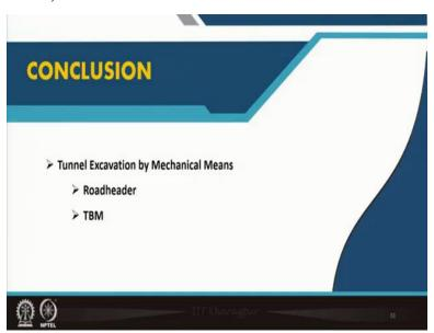
So, so actually today we have learnt about the tunnel excavation by mechanical means. There are two equipments like roadheader and TBM. Roadheader is obviously, as I have mentioned that when means relatively less costly means as compared to the TBM. TBM is quite huge machine, so costly and operating cost is quite high.
