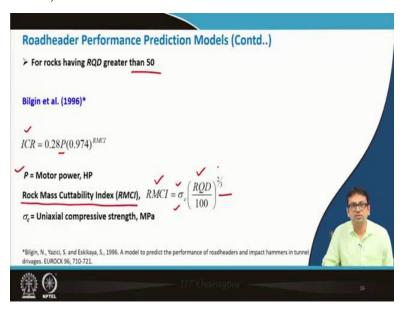
Now for rocks having RDQ value greater than 50 actually, then Bilgin et al. (1996) they have given some equation like ICR, the same thing instantaneous, ICR is instantaneous cutting rate so ICR is equal to 0.28 p into 0.974 to the power RMCI, now what is this RMCI? Obviously, the p here you can see p is the motor power in horse power HP, what is the RMCI? The full form is rock mass cuttability index.
