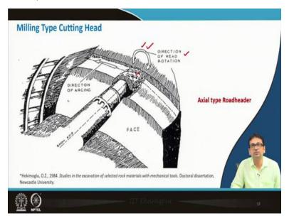
So, now milling type cutting head that is important we should understand at least these terms or what do they mean actually. You see here look at, so milling type cutting head is like your cutting head is here as you can see over here and direction of head rotation. So basically, it will rotate in this way this cutting head, so and it will obviously move forward there is no doubt about that in this way, so it will keep on rotating like this as you can see from here.
