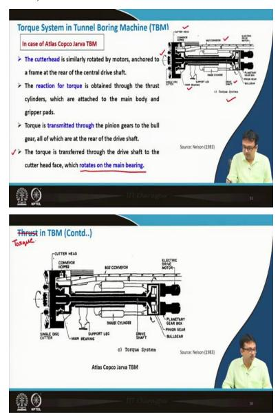
Now in case of, this is for the torque system in the Atlas Copco Java TBM, sorry here it should be, the torque, this is not for this, this is for the torque, torque in TBM we are discussing about that. So now, torque system in TBM in case of Atlas Copco Java TBM so same diagram as it is shown in previous slide, the cutterhead similarly rotated by motors anchored to the frame at the rear and the central drive shaft.
