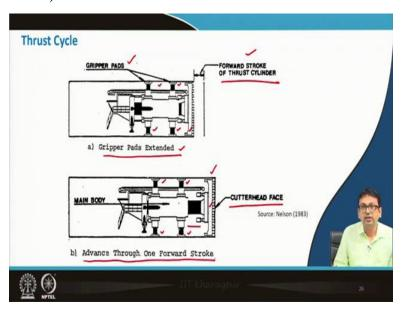
Now this is very nice, you see, pictorial representation of this thrust cycle. What is happening? forward stroke of thrust circle as you can see now this is gripping pads extended. Now next stage, what is done?
