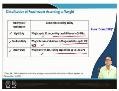
Now classification of roadheader according to weight; so with this is by Tucker (1985), so what is this way it is divided like light duty, medium duty, heavy duty. Now, the weight in case of light duty roadheader is 30 ton, medium rate is 34 to 45 ton and heavy duty is more than 45 ton. Now very important thing is cutting capability up to 70 mega Pascal in case of light duty.
