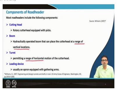
Now, components of roadheader, so most roadheaders include the following components like; cutting head
