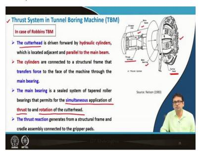
In case of this Robbins TBM, the cutter head as you can see here clearly mentioned that this is our cutter head. The cutter head is driven forward by hydraulic cylinders. Therefore, you can see that it is regarding the thrust system in TBM, so in case of Robbins TBM this for this third system you see third cylinders are there.
