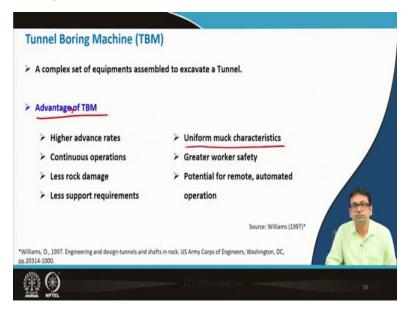
Tunnel boring machine is actually a complex set of equipments assembled to excavate a tunnel. Now, there are some advantage of TBM tunnel boring machine in short we frequently call it as TBM, so basically some of the advantages like higher advance rates. Therefore, it is quite fast and continuous operations can be performed. It has less rock damage; obviously surrounding rock will not be damaged that much as compared to the drilling and blasting as we can understand.
