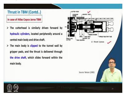
Now in case of Atlas Copco Jarva TBM, the same diagram only shown over here; the cutter head is similarly driven forward by hydraulic cylinder located peripherally around a central main body and drive shaft and the main body is clipped to the tunnel wall by gripper pad. So, this gripper person actually for that purpose the main body is clipped to the tunnel wall by gripper pads and the thrust is delivered through the drive shaft which slides forward within the main body.
