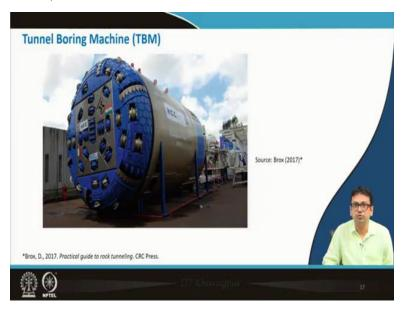
Now the analog means the next one is tunnel boring machine which is like you can see the picture; huge equipment, you can understand it is a huge equipment and obviously extremely effective useful equipment and throughout the world. It is used like frequently for tunnel construction. Only thing is you see as it is very big, so it is costly as well as operating cost is also quite high.
