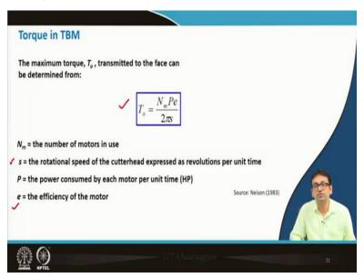
Now torque in TBM; the maximum torque  $T_0$  transmitted to the face can be determined from this simple equation;  $T_0$  is equal to  $N_m P e / 2\pi s$ . Now  $N_m$  is the number of motors in use, s is the rotational speed of the cutter head expressed as revolutions per unit time, P is the power consumed by each motor per unit time, this should mean horsepower HP and e is the efficiency of the motor, so based on that one can find out the maximum torque  $T_0$ .
