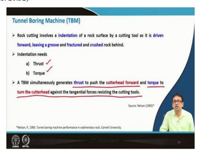
Now, again what we can say that rock cutting involves an indentation of a rock surface by a cutting tool as it is driven forward leaving a groove and fractured and crushed rock behind. Now indentation needs two thing; thrust and torque. Now, a TBM simultaneously generates thrust to push the cutter head forward and torque to turn the cutter head against the tangential forces resisting the cutting tool.
