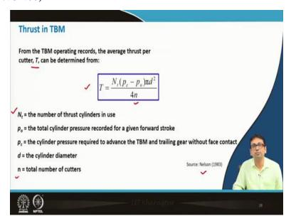
Now from the this TBM of this means let us try to learn see some expressions for this thrust per cutter. What is stated from the TBM operating records the average thrust per cutter that is t can be determined from this equation, so this you can find in obviously in this Nelson (1983) as the previous diagram is also from Nelson (1983) as it is shown and the reference is provided earlier, I can show you reference also yeah.
