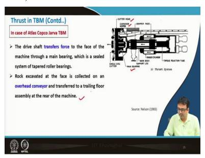
We can say the drive shaft transfers force to the face of the machine through a main bearing as we can see over here. The drive shaft transfers force to the face of the machine through a main bearing which is a sealed system of this tapered roller bearings and rock excavated at the face is collected on an overhead conveyor as it is shown over here.
