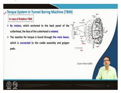
In case of Robbins TBM, by motors, you see again the, this Robbins TBM torque system you see here look at here, so torque you can clearly means this is for the torque and earlier one was for thrust. So by motors which anchored to the back panel of the cutter head, the face of the cutter head is rotated. The reaction for torque is found through the main beam which is connected to the cradle assembly and gripper pads actually.
