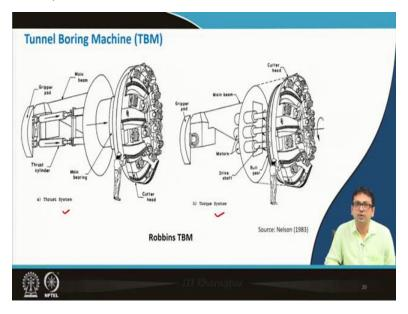
Now, there are different TBMs available, so this is actually the picture of the Robins TBM, Robins TBM there you see the, this is the thrust system is shown over here and torque system is shown over there in the Robbins TBM, Robbins tunnel boring machine.
