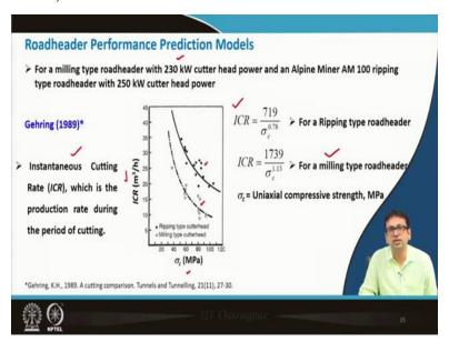
Now, roadheaders this performance prediction models, so for a milling type roadheader with 230 kW cutter head power and an alpine minor AM 100 ripping type roadheader with 250 kW cutter head power. Gehring (1989) gave some like formula or expressions for that based on the data actually, so one term was introduced like instantaneous cutting rate ICR, which is the production rate during the period of cutting.
