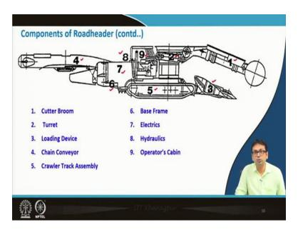
Now this is different components of roadheaders, again what I have mentioned actually, so one; here you can see 1 is for cutter broom. This cutter broom is there right so as you have seen over here cutter head like so here that is what you can see from here. Then turret, then loading device, 2 means turret you must have understood and 3 is loading device as I mentioned 4, which is chain conveyor.
