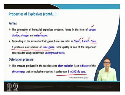
Next property is fumes. This is very important. So, basically, the detonation of industrial explosives produces fumes in the form of carbon dioxide, nitrogen, and water vapor. Now depending on the amount of toxic gases fumes are rated as class 1, 2 and 3. Now what does it mean?
