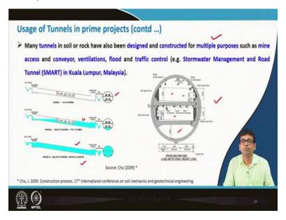
Now a days many tunnels in soil or rock have also been designed and constructed for multi-purposes such as mine access and conveyor, ventilation flood and traffic control.
