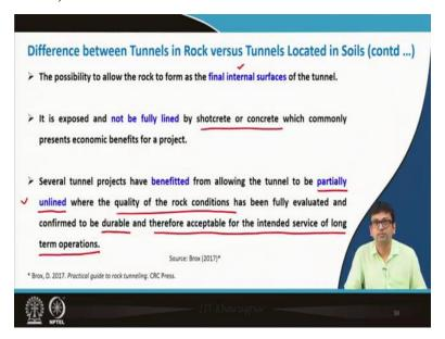
The possibility to allow the rock to form as the final internal surface of the tunnel; whereas, in soil, some liners are provided. Generally, concrete liner or shotcreting is applied. We will discuss about these terms later obviously.
