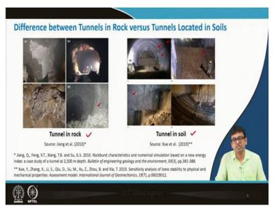
Figure shows the tunnel in rock and the tunnel in soil. Clearly, the rock surface can be seen. Whereas, in case of soil, some concrete liner is provided because soil will not be able to stay there means in its own, it may fall.
