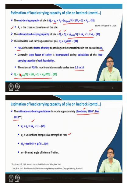
So, the final expression for the end bearing capacity of pile will be  $Q_p = q_p \times A_p$ . Now,  $q_p = q_u \times (N_{\varphi} + 1)$ . Now,  $q_u = q_{u(\text{design})}$ . So,  $q_{u(\text{design})} = q_{u(\text{lab})}/5$ .
