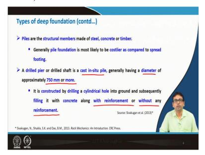
Piles are the structural members made of steel, concrete or timber. Now, generally, pile foundation is most likely to be costlier as compared to the spread footing. It is quite obvious as the piles are maybe of 10 m, 15 m, 20 m, 30 m of length. Now, the second category, a drilled pier or drilled shaft is a cast in-situ pile generally having diameter of approximately 750 mm or more.
