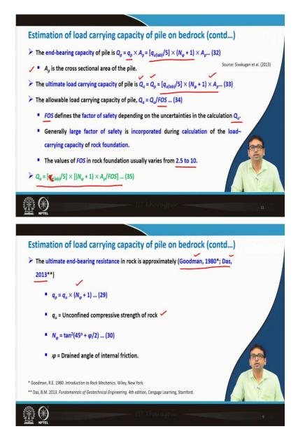
Now, based on this, let us take a problem to clear the doubts. The estimation of load carrying capacity pile on bedrock. So, here is the problem statement given that a pile of diameter of 50 cm. The length is 15 m passes through the highly jointed and weathered rock mass and rests on a shale bed. For shale, laboratory unconfined compressive strength is equal to 40 MPa.
