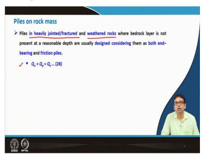
Now, piles are on the rock mass. So, piles in heavily jointed or fractured and weathered rocks where bedrock layer is not present at the reasonable depth are usually designed considering them as both end bearing and friction piles.
