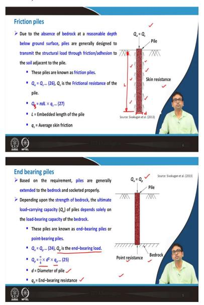
Now, the friction piles. Due to the absence of bedrock at a reasonable depth below ground surface, piles are generally designed to transmit the structural load through friction or adhesion to the soil adjacent to the pile which is also known as the skin resistance. So, that is the frictional resistance.
