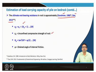
Now, the ultimate end-bearing resistance in rock is approximately as per these two references (Goodman 1980 and Das 2013) is  $q_p = q_u \times (N_\varphi + 1)$ , where  $q_u$  is the unconfined compressive strength of the rock and  $N_\varphi = \tan^2\left(45^\circ + \frac{\varphi}{2}\right)$ , where  $\varphi$  is the drained angle of internal friction. So, the equation is as per Goodman 1980 and Das 2013.
