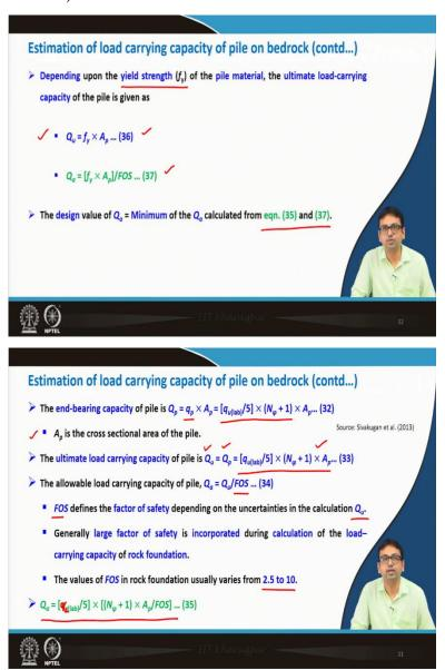
Now, depending on the yield strength  $(f_y)$  of the pile material, the ultimate load carrying capacity of the pile is given as  $Q_u = f_y \times A_p$  which is governing here. As it has been mentioned earlier, for good quality rock (generally), the capacity calculated from the strength of the rock is higher than the yield strength of the pile material.
