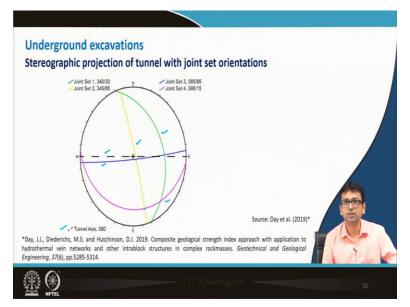
And you see, same way for stereographic projection of tunnel with joints set orientation you see there are 4 joint sets we can clearly notice. So, this is 1, 2, 3 and 4. So, now, they are intersecting like here, one intersection here, here, here these are different intersections and now also that you see tunnel axis is shown within this. So, tunnel exit is shown with this.
