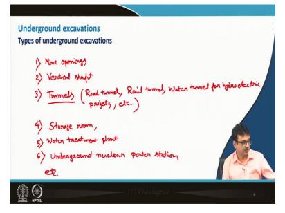
So, now the type of underground excavations. So, we know that there are different types of underground excavation some of them let me write down over here maybe number 1 we can write it as like mine openings, this is very common in the mining industry. Then vertical shafts I will show you some diagram also for vertical shafts. Vertical shafts are also quite frequently required to construct. Other than that the tunnels are the most important one of the underground structures.
