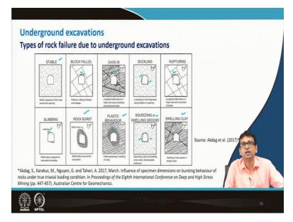
Now, types of rock failure due to underground excavation. So, let us see this nice picture. So, from here you can clearly understand you see here in this case it is quite stable. But, you see here you see the block failure is occurring whereas here cave-in then here you see the sides are if you look at here, here buckling then here rupture has occurred then clearly you see that cracking has developed.
