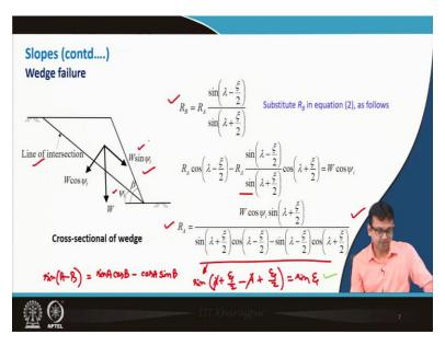
So, now RA and RB are here with us, now factor of safety suppose our cohesion for c suppose equal to 0, so if it cohesion is there then also it is no problem we have to simply obtain the area of that plane in A plane and B plane and you have to multiply that with your cohesion that will give that resisting force it will further increase, anyway if we consider simply c 0, so then our equation becomes RA plus RB they are nothing but as I have mentioned RA and RB are what?
