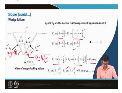
Now, resolving this RA, this forces RA and RB into components of normal and parallel to the direction along the line of intersection, along the line of intersection we get a couple of equations, so they those are nothing but the force equilibrium equation, simply we just look at this diagram and let us go for the force equilibrium.
