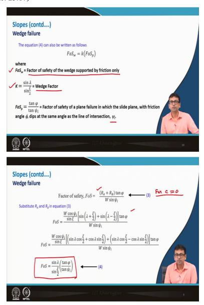
Now, this equation may have been given name like 4, this is the ultimate equation but anyway we will just introduce two more terms over here. So, this factor of safety suppose W subscript if we write and if we write a k factor of safety p, so what are they?  $FoS_w$  is ultimately the desired thing which is the factor of safety of the wedge, so factor of the safety of the wedge supported by friction only as we have considered c is 0.
