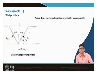
Now, this is nothing but view of the wedge looking at the face and it is very simple here RA and RB are nothing but the normal reactions provided by plane A and plane B.
