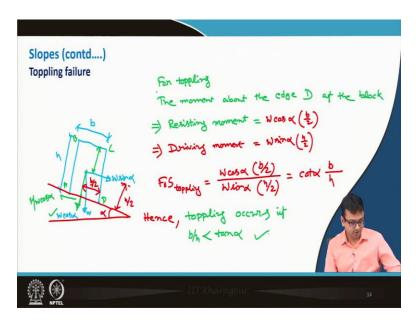
So, in case of toppling failure just quickly let me draw this diagram that is very important try to draw it now, this is my suppose  $\alpha$  angle and suppose this is the block. And so b and h so what we can see from here that this is suppose W, now Wsin $\alpha$  and this is normal, so Wcos $\alpha$  and you can consider that here  $\mu$ Wcos $\alpha$  exactly.
