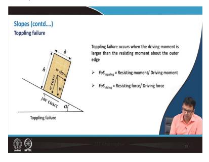
So, toppling failure means if we simply draw this diagram, this free body diagram from there we can very easily understand the mechanics behind this. So, one thing is this toppling is associated with sliding also, so that is also one thing we will notice over here. So, the toppling in some is associated with the sliding also.
