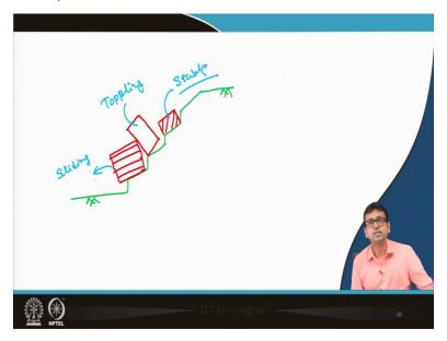
So, now small diagram where I will show you in pictorial diagram to give you some idea about this type of failure modes. This is ground surface, now what may happen, this is toppling, this block, whereas this one is sliding, so this is neither topping nor sliding.
