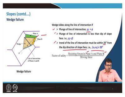
So, again let us go back here, so plane A is providing suppose normal reaction RA and plane B is providing the normal reactions suppose RB.
