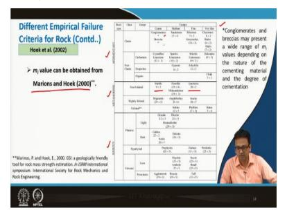
Now for finding out  $m_i$ , in 1997, a table was given different types of rock like sedimentary, metamorphic, igneous but again Marions and Hoek in 2000 modified it and they have given a new table which is a little different from the previous one. In this table for different rocks  $m_i$  can fall in a range.
