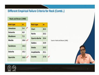
Refer to the tables given in slide 6 of this lecture for m values of different types of rock so by giving these as the input you can utilize the equation of Hoek and Brown for any numerical calculation.
