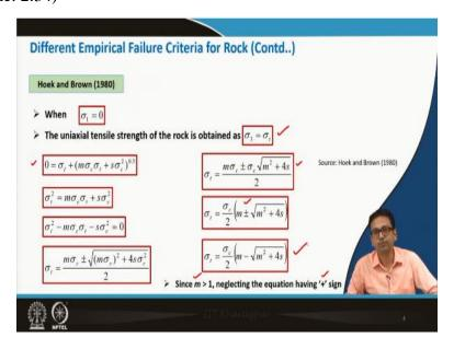
Now for further discussion when  $\sigma_1 = 0$ , the uniaxial tensile strength of the rock is obtained as  $\sigma_3 = \sigma_t$  or by further simplifying the previous equation
