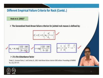
Hoek et al 2002, is the most widely used criterion as it takes into account almost all the flaws that were there in the previous version. So, the generalized Hoek Brown failure criteria for jointed rock masses is defined by
