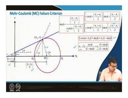
Now if we again look into the figure, three points- the point where the failure envelope cuts the  $\sigma_n$ - axis at an angle  $\phi$ , point where the envelope meets the Mohr circle and point O. These three points make a right angled triangle. Using this triangle, we can observe that-
