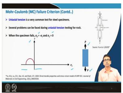
Uniaxial tension is a very common test for steel specimen, but in case of rock there may be some difficulties regarding gripping. Now fundamentally in this test, only the uniaxial tension is
