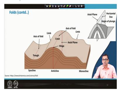
So, next is that we will discuss about the different components of a fold. So, if it is a typical diagram of a fold, so you can see this plane is called as the 'Axial Plane'. This line is called the 'Axis' of the fold. Likewise, it is also the 'Axis' of the fold. For this pattern, the folds is concave upward; this is concave downward button for that. This is the 'Axis' of fold; this is also the 'Axis' of fold.
