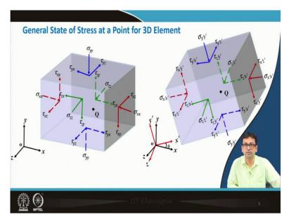
So, for the generalized state of stress at a point for 3D element, the stresses will be as per the first diagram which we have seen in the previous lecture and for an arbitrary orientation of the element, the stresses will be as per the second diagram.
