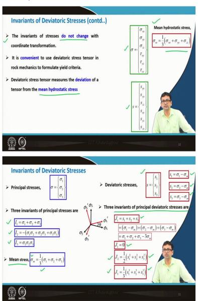
So now, let us discuss about this invariants, so what are the invariants? The invariants of stresses do not change with the coordinate transformation, which is the biggest advantage of using these invariants. We will see in the latter module that when you present the failure criterion, then we will try to use these invariants, so that it should not be dependent on the coordinate transformation. It is very important that the invariants of stresses do not change with coordinate transformation.
