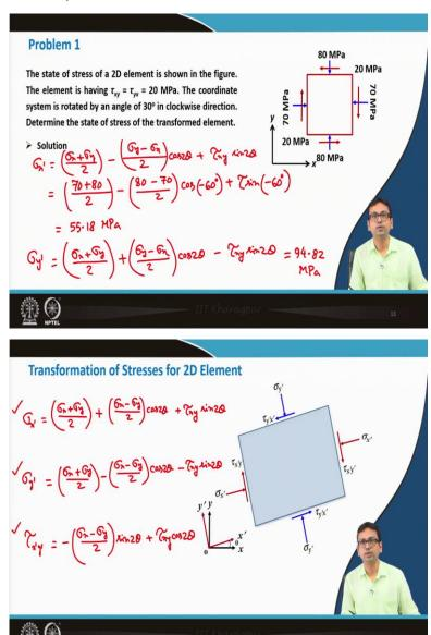
Now, let us solve a small problem with that will conclude our today's class. So, it states that the state of stress of a 2D element is shown in this figure. The element is having  $\tau_{xy}$  or  $\tau_{yx}$  is equal to 20 MPa. The coordinate system is rotated by an angle of 30° in clockwise direction. Determine the state of stress of the transformed element.
