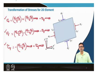
What are the expressions of  $\sigma_{x'}$ ,  $\sigma_{y'}$ , and  $\tau_{x'y'}$  in terms of the known stress components like  $\sigma_x$ , ,  $\sigma_y$ , and  $\tau_{yx}$ ? It can be obtained by doing a simple small derivation.
