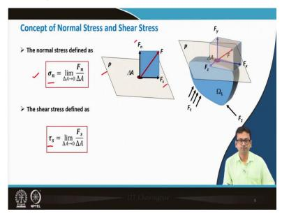
So, form the figure, we can see that this is the P plane and  $\Delta A$  is the small area, and F is the resultant force. Now, it is resolved into two components, one is the normal component,  $F_n$  (in the normal direction), i.e., normal to this  $\Delta A$  or normal to this plane P and the other one is the shear component,  $F_s$ .
