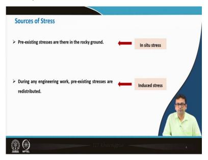
The pre-existing stresses are there in the rocky ground, which is mainly the in-situ stress. Other than that, during any engineering work, pre-existing stresses are redistributed. As a result, the induced stresses come into the picture.
