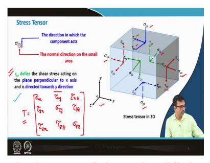
Now, let us learn about the stress tensor. So, let us see the small 3D element. What are the stresses will act in the element? If this is the coordinate system, we will have one normal stress and two shear stresses,  $\sigma_{xx}$ ,  $\tau_{xz}$ , and  $\tau_{xy}$ . Now, here you can see the suffix xx or xy. What do they represent? let us try to understand.
