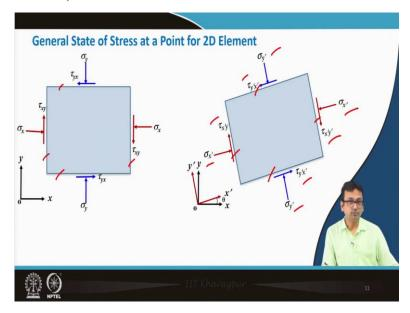
Now, let us see the general state of stress at a point for a 2D element. This side and this side are parallel to x-axis and this and this sides are parallel to y-axis. Now, the coordinate system is rotated by an angle  $\theta$ . Thus, this side is making an angle  $\theta$  with the x-axis, similarly, this side is also making an angle  $\theta$  with the x-axis and these sides are making also  $\theta$  with the y-axis.
