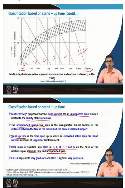
To understand the classification system better, refer to the figure in the slides- the y-axis is the active span and the x-axis represents stand-up time. A represents very good rock means, it will have more stand-up time and class G signifies very poor rock.
