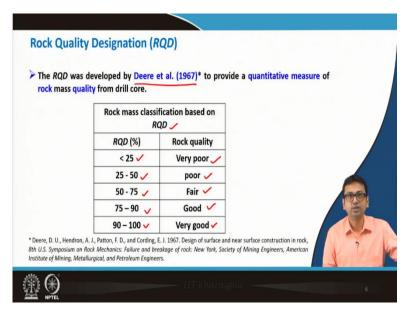
Now we will see the RQD, rock quality designations and the classification based on this. This is a very simple way of classifying the rock mass and RQD was developed by Deere et al. in 1967 to provide a quantitative measure of rock mass quality from drill core. We have already seen how to find out RQD.
