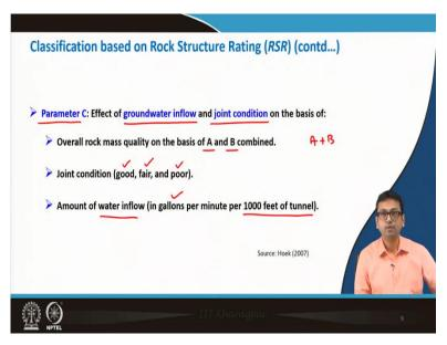
And now, the third parameter that is parameter C. For that the RSR table 3 we have to use and this is related to groundwater, joint condition and parameter A and B. So, now here first we have to find out A + B. We will get A and B from RSR table 1 and RSR table 2.
