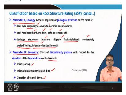
Now, this parameter A is corresponding to the geology. General appraisal of geological structure on the basis of few things, first very important thing is rock type origin.
