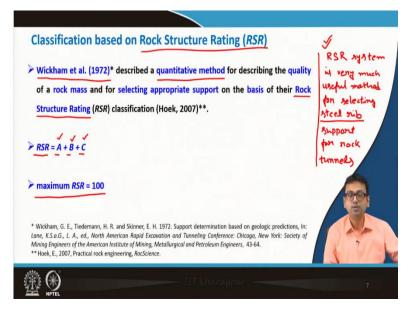
Now we will discuss the classification based on rock structure rating RSR. This rock structure rating concept is very useful. This classification system is very useful for selecting steel ribs. Steel ribs support when we are designing a tunnel in the rock.
