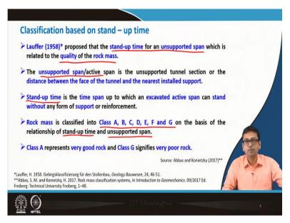
Let us discuss another classification system that is based on stand-up time. Lauffer 1958 proposed the stand-up time for an unsupported span which is related to the quality of the rock mass. What is an unsupported span or active span? The unsupported span or active span is the unsupported tunnel section or the distance between the face of the tunnel and the nearest installed support.
