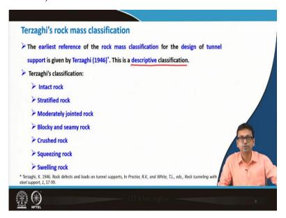
Terzaghi's rock mass classification. The earliest reference of the rock mass classification for the design of tunnel support is given by Terzaghi in 1946. It is a descriptive classification.
