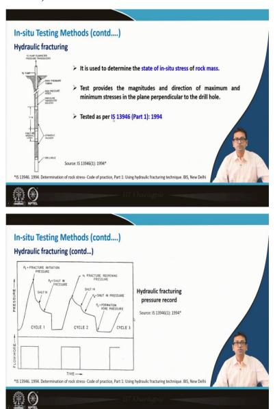
Now, hydraulic fracturing just now, we have discussed. So, similar type of arrangement, you see two packers are there, this portion isolated. Now, what is done here and why it is done it is used to determine the state of in-situ stress of rock mass. So, the test provides the magnitude and direction of maximum and minimum stresses in the plane perpendicular to the drill hole.
