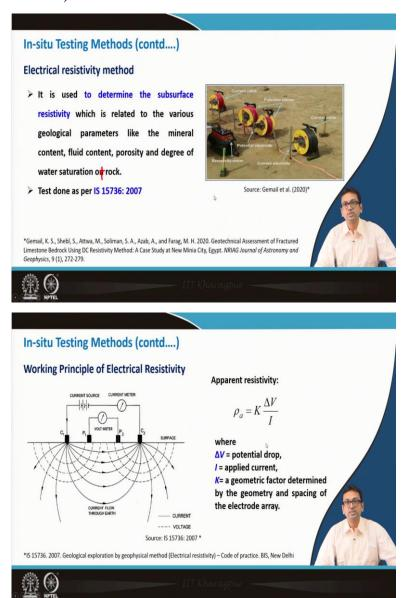
Now, briefly the electrical resistivity method. So, this is used to determine the subsurface resistivity which is related to the various geologic parameters like the mineral content, fluid content, porosity and degree of water saturation on rock. So, the test is done as what IS 15736: 2007. So, these are the different electrodes are shown over here current electrodes and potential electrodes.
