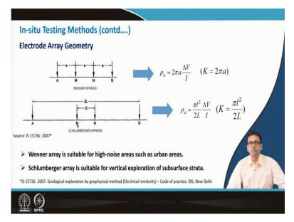
Now, then, we define different types of array, popular one is Wenner Spread where you see that these are A, B at the current electrodes and M, N at the potential electrodes. So, you see the distances are a, a, a, whereas Schlumberger Spread here you see if this is 2L and this l and this is two L. So, here these differences are a, a but where it is not fixed. So only thing is the distance from here to here and the distance from here to here are fixed.
