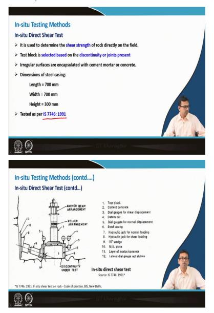
So, In-situ direct shear test very much similar to the direct shear test we conduct in our laboratory only the thing is here, the equipment is definitely quite big in size. And, let me show you that just the diagram, I think that will be first let me show you the diagram then I will come back over here. So, this is the pictorial representation of the direct shear test apparatus for conduct In-situ testing.
