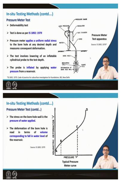
Now, next is pressure metre test. So, this is again for conducting pressure metre test, one should follow IS 1892: 1979. Now, what we can say this is also a deformability test, so deformability of rock mass can be found out by conducting this test and this is as per IS code as I have stated. Pressure metre applies a uniform radial stress to the borehole at any desired depth and measures consequent deformation.
