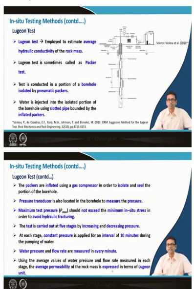
Now, remember when we have discussed about the permeability of rock mass then we have discussed that there are different tests for obtaining the coefficient of permeability hydraulic conductivity of rock, means intact rock in the laboratory or the rock mass in the field among them. One of the very important tests is Lugeon test and which is also called as the packer test. So, here you can see the schematic diagram.
