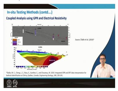
And now, if you see use the both GPR and electrical resistivity method then that can be a great thing. So, with the help of the GPR you may get this type of picture and whereas, using electrical is you can get this type of picture. So, combining these two, you can understand in a better way of definitely or obviously you can perform some of the verbal study also to get a better and complete idea about the subsurface condition.
