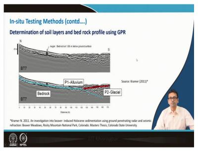
So, finally, this may give you a wide area means you can get this type of GPR obtained picture you can get. Now, in order to verify whether your GPR data is correct or not. So, you can perform some borehole tests to get what type of samples are there.
