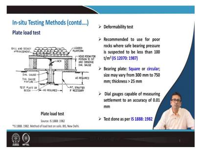
So, plate load test it is about this you have learnt in your soil mechanics. So, similar to that similar setup, as you can see over here that this is the test feed, if this is BP the size of your plate of which you are conducting that test. So, if it is BP then generally this dimension should be 5 BP because people will be there to conduct the test it should be, they should have enough space to do the activities freely.
