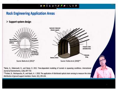
Now, supports system design. Suppose, if we see these two pictures, these are for tunnels. You may find that after carrying out the numerical analysis, the tunnel is not stable enough means under the loading, whatever loading will come there, because of the loading it may fail or if some earthquake comes it may very easily collapse.
