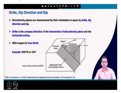
Now, before further continuing with these faults, let us discuss about three essential parameters - they are strike, dip direction and dip. They are very important as these things will be found to be useful when we will design suppose a tunnel or a foundation or any structure in rock.
