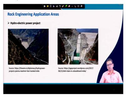
Then hydroelectric power project, this is actually one of the very important civil engineering structure and they are mostly constructed in the hilly terrain, so like the right side picture is of the Tehri dam in Uttarakhand. So, for designing hydroelectric power projects, where you have to construct huge dam, there your knowledge of rock engineering will become very essential actually.
