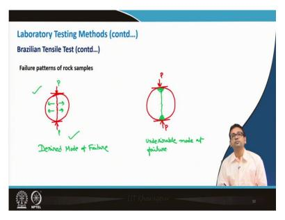
Now, let us see, what the different failure patterns of rock samples are in case of the Brazilian tensile strength test. P is the applied load to the sample as shown in the figure. So, what is expected there that this kind of crack will develop means under this P loading, the tensile forces developing in this direction and because of that the sample is failing. So, this is the expected failure pattern.
