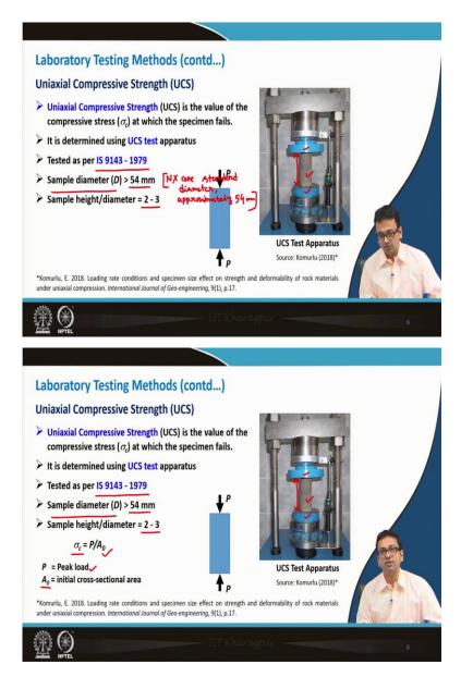
Now, let us start discussing about another very important test, about which we have spent a good amount of time in our previous module also, but let us see what the basic test procedure is. So, uniaxial compressive strength (UCS) is the value of the compressive strength at which specimen fails. Now, it is determined using this UCS test apparatus and the IS 9143 - 1979 can be followed to conduct this test.
