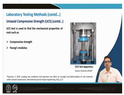
So, the UCS test is used to find the mechanical properties of rock such as compressive strength, Young's modulus, Poisson's ratio, and etcetera.
