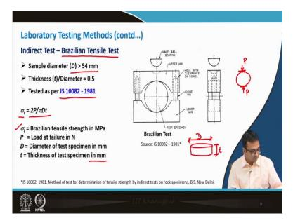
Now, another test procedure we will discuss here that is called as the indirect tensile test, also known as the Brazilian Tensile Test, so it will give indirectly the tensile strength of the rock sample. In the case of direct tension test, we are applying tension directly and getting the tensile strength by stretching the sample or specimen.
