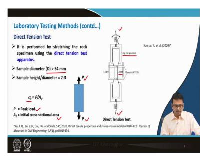
So, now, let us discuss about the tension test. So, the first one is the direct tension test. From the diagram, you will understand clearly why it is called as direct tension test. And since we are discussing a direct tension test, so we will also discuss here about the indirect tension test also. So, firstly, let us see the direct tension test. It is performed by stretching the rock some the specimen using the direct tension test apparatus.
