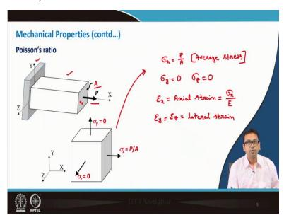
Now, one important thing is Poison's ratio. It is very important to discuss because that gives us a lot of information. Like if we first think about suppose this is a maybe a beam and fixed at this point here is the beam. Now a load P is acting along x axis only and in y and z direction there is no force acting, let us consider the area of this surface is A.
