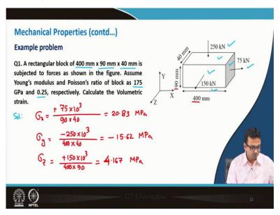
Now, with this idea, let us take a small problem the problem says the a rectangular block of 400 mm by 90 mm by 40 mm is subjected to forces as shown in figure. As you can see here 75 kilo newton, here tensile force there it is 250 kilo newton compressive force again here Z direction 150 kilo newyon tensile force is acting. Assume Young's modulus and Poison's ratio of block as 175 Giga Pascal and 0.25 respectively calculate the volumetric strain.
