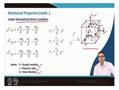
So, now, if I consider a case like this generalized case were not only the normal stresses but also the shear stresses are acting. So, that becomes actually in true sense of the generalized stress condition and under there not only these 3 equations what we have just have derived actually, along with this we need to also consider these 3 equations also.
