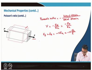
Now, let us see next diagram. Yes, so, this is what actually what I was telling, if I apply a force P here so then means, if it is initially suppose of this shape, then because of the application of load, what will happen it will elongate and it's in y and z direction it dimension will reduce. So, that is very well understood. So, that is nothing but called as the Poison's effect and from there this Poison's ratio comes to the picture.
