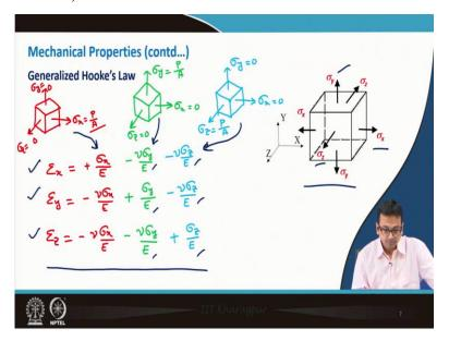
So, here just first you consider only the keys of only you have applied the force in the x direction. So, suppose just one by one let me take I think that will be easier for you to understand. So, if this is the case where only I have applied I have this only so it is sigma x is equal to suppose P by A average stress and here and here they are maybe 0 and 0, then if I want to write down my epsilon x that is definitely nothing but this plus sigma x by E.
