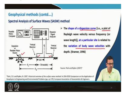
Now, just last 1, 2 things, they are nothing but I just have told you. Another instrument is, method is called as Spectral Analysis of Surface Wave method. So, here surface wave is utilized for this purpose, measurement. So, you see there is a source, then, 2 receivers are used, vertical receivers are there and this is my data acquisition system, it is a delicate instrument means relatively little more costly but very useful, nowadays very popular.
