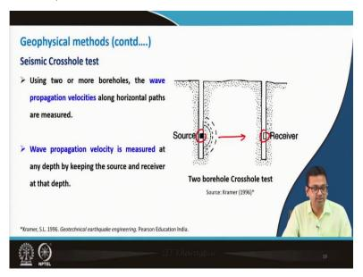
Now, seismic crosshole test, quickly we will discuss about this. In means, there maybe we can using two or more boreholes, wave propagation velocities along horizontal path you see this path it can be obtained, measured. So, here it is shown for a 2-borehole cross hole test. So, here as you can see source is here, receiver is here and the wave propagation velocity is measured at any depth by keeping the source and receiver at the same depth actually.
