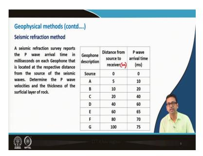
Now, this is a small problem. A seismic refraction survey reports the p-wave arrival time in milliseconds on each geophone that is located at the respective distance from the source of the seismic waves. Determine the p-wave velocities and the thickness of the surficial layer of rock. After conducting the seismic refraction test these are the data we will get. So, geophone descriptions like source A, B, C, D, E, F, G and corresponding distance from source to the receiver.
