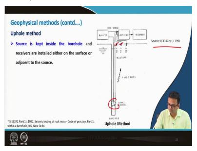
So, on the other hand uphole test, what uphole method what we do? The as again this also you will get in same IS code so, source is kept inside, you see? The source is here and inside the borehole and receivers are installed either on the surface or adjacent to source. So, this is the, here the receivers are placed.
