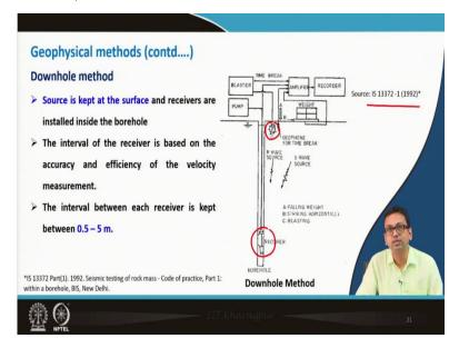
And downhole method is very simple, this is the arrangement. See for this I am we can get the guideline from the IS 13372 Part 1 1992. So, this is for downhole method. So, source is kept at the surface and receiver are installed inside the borehole. So, you see there is the source at the ground surface and receivers like here. So, the interval of the receiver is based on the accuracy and efficiency of the velocity measurement.
