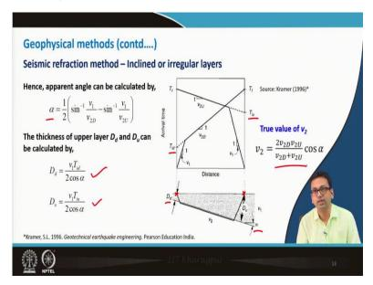
So now, for that some expressions are available. So, obviously, different researchers have developed this I am not going to those derivations. So, first one is the opponent angle. So, apparent angle can be calculated by this equation this. So, alpha is my apparent angle as it is shown over here. So, this is half sine inverse  $V_1$  by  $V_{1D}$  minus sine inverse  $V_1$  by  $V_{2\underline{U}}$ . Now, what are they?
