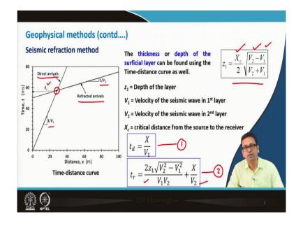
Now, you see another thing I will show you, this thickness or the depth of the surficial layer can be found using the time distance curves as well. So, time distance curve is nothing but in Y axis will show time, X will show distance. Now, distance is nothing but the distance between the source and the receiver and then the same expression shown Slide 6.
