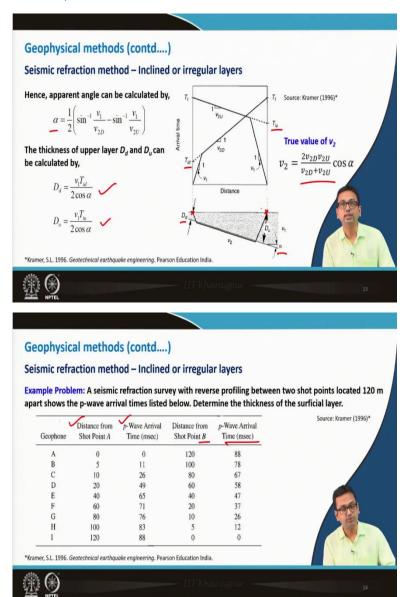
So now, let us take a small problem and make our concept clear. So, a seismic refraction survey with reverse profiling. So, this is called reverse profiling. So, once you will, first you will keep your source at a location and at geophone or receiver at one location and then at those locations only again you will just interchange the position means your first source here, receiver here then source here, receiver here.
