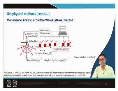
Similarly, that was Spectral Analysis of Surface Wave, SASW, another one is Multichannel Analysis of Surface Waves MASW. This is also based on that surface wave principle means using that we tried to get the other seismic velocities and we tried to finally find out the profile of that particular area, what type of profile is there that we can get.
