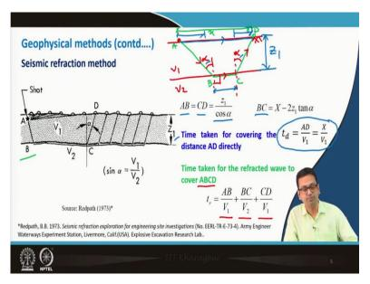
So, let us go to our next slide. So, here you see this is the initial diagram as we have seen in our previous class also. The source is point A and from there this ray is getting reflected in layer 2 and this  $\beta = 90^{\circ}$ , here, this is our  $\alpha$  and here also  $\beta = 90^{\circ}$  then again  $\alpha$  and it is reaching at D. On the other hand, direct waves are also there, so, direct wave is going like this.
