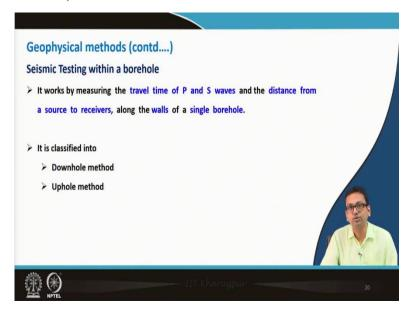
Basic idea you can get. Likewise, there is another type of test which is means within a borehole it is done actually. So, source and receiver means, it works by measuring the travel time of P and S waves and the distance from a source to receiver along the wall of the single borehole. So, both are there in the single borehole, you can do it. So, classified into categories downhole method, uphole method
