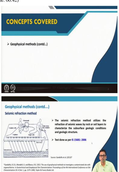
In our previous class, we started discussing our seismic refraction method, before that, we have completed seismic reflection method in detail and solved a example problem also. So now, we will continue our discussion related to seismic refraction method.
