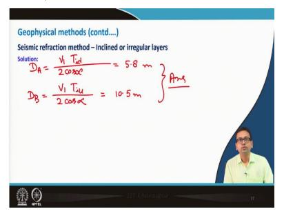
So, my DA will be  $V_1T_{id}/2\cos\alpha$  and DB is equal to  $V_1T_{iu}/2\cos\alpha$ . So, if you place these values you should get it a 5.8 metre and this one is 10.5 metre. So, these are your answers. So, you see even for incline ground also you could able to get it very easily.
