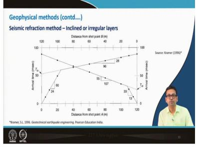
So, we have plotted this for the direct wave and these are for refracted wave and these are nothing but the slope some numbers are provided here. So, for quick reference these are given. So, from here as we know this is nothing but as we have seen over here in this diagram. So, this one is  $1/V_1$ , this is 1/2,  $1/V_{2D}$ . This is again  $1/V_1$  this is  $1/V_{2D}$ . So, those are the values are provided here for our quick reference now.
