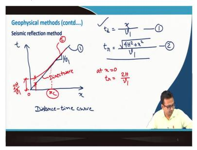
Referring to the diagram in slide 5, If I consider this direction it is x and this direction it is t, this is distance time curve we are trying to plot. So, if I plot this one, we will get a straight line passing through the origin. And, the slope of this plot will be 1 by v1.
