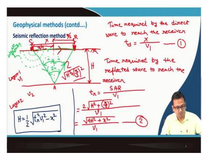
What is the idea behind this? Referring to slide 4, there is a source and at a distance X, your receiver, the geophone is present over there and there is the ground surface. There are two layers - layer 1 and layer 2. Suppose velocity of seismic wave at layer 1 is  $V_1$ , and at layer 2 it is  $V_2$ . Now, one thing what will happen? One is, directly this will go from source to receiver.
