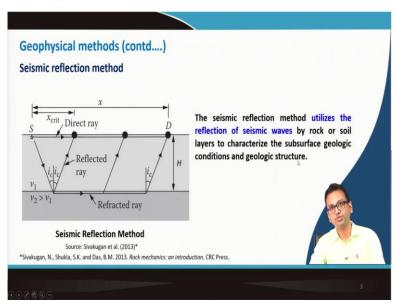
As discussed in the previous class, there are different methods like seismic reflection method, refraction method, cross-hole method etcetera. So, out of those things, today we will discuss about the seismic reflection method. In the diagram in slide 3, you can see that if there is some source from where seismic waves are generating, then if we place some receivers at certain distances, like receivers means mainly the geophones are used for that purpose.
