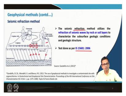
Now, the second one which is extremely useful and for this instrumentation, the curve is a little bit more sophisticated, but it is very useful in determining the thickness of maybe see with the help of the reflection survey in general you will get the thickness of only the upper layer. Now, there maybe you may be interested in knowing maybe thickness of 5 layers or 10 layers.
