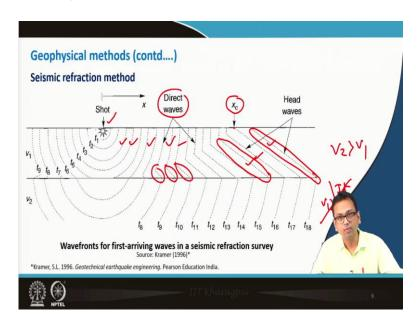
So, let us see how to do that. Suppose this is the source, now after hitting, seismic waves are generated. So now, these are nothing but the wave fronts as I have stated. So, this is layer 1, layer 2, now, at layer here this is going like this, but then when it is reaching at the layer 2 you see these portions have started developing and ultimately these are becoming very much predominant.
