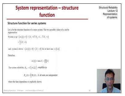
Let us define the structure function for the pure series system which we have looked at in the past. So, the system as we know that it is up only when all the elements are up. So, we can express the event of alpha equals one in terms of all the X's as you see on the screen and likewise alpha is zero when at least one of the element states is 0. So, then we could express alpha in terms of X's in 2 equivalent ways.
