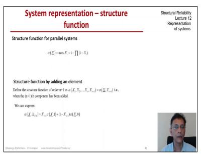
The structure function for the parallel system would going through a similar logic would be the maximum of all the X's even if one of them is one then the system is up and which could be given in terms of one's complement of the product of 1 - X is there is one useful way of expanding the structure function of a system when you add one element. So, it is basically using a partition approach that we have done before.
