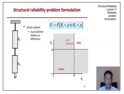
Our next problem concerns a 2 unit system or 2 element system in series. So, there are 2 cables hanging from the ceiling subjected to a point load p and let's see how we set the problem up in terms of the mechanical behaviour of the units or the elements they could be ductile on the one extreme or brittle on the other extreme. But it so, happens that when you have a serious system like that it makes no difference to the failure domain as we will see.
