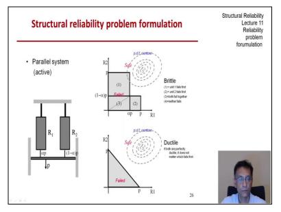
So, we have now a parallel system and later we will see that this arrangement is called an active parallel system. So you have the load p, R 1 and R 2 is connected in parallel it is not necessary that the load be shared equally between the 2 elements. Let us say the loads are shared as in terms of alpha and one minus alpha ratio. So, R 1 carries alpha p and R 2 carries 1 minus alpha p. So, what would be the failure domain or the failure set when the behaviour is brittle.
