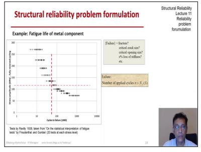
As the first example on how to set up a reliability problem let us take a look at these fatigue tests done way back in 1938. As I was saying yesterday that fatigue was one of the oldest problems studied in reliability. So, these tests were conducted on 20 samples each at each stress level and what you see here are 10 stress levels. So, those markings are the fatigue life of each component tested at the respective test levels.
