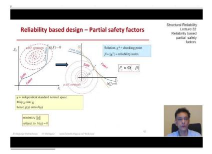
And in the end the objective is to in this u space find the minimum distance from the origin to the transformed limit state surface which is h of u = 0 and so this is the mathematical description of the problem, we minimize the distance from the origin to the line or the surface h = 0 and the solution is U star and that minimum distance is beta the reliability index.
