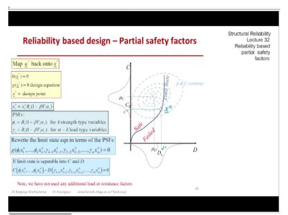
Now we can then with these partial safety factors rewrite the limited equation that g of x star = 0 at the design point in terms of these partial safety factors and the nominal values. And this actually takes us closer and closer to a design equation. So, even if we stopped here we would have an equation involving the partial safety factors, the nominal values and if the
