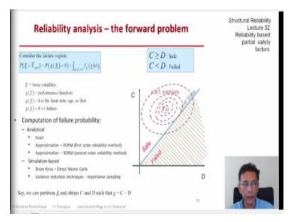
We have basic variables X and we have the limit state g X = 0 the limit state equation, so that g X negative implies failure. And we have spent a good amount of time discussing how to compute the failure probability using analytical methods, approximate methods FORM, SORM, Monte Carlo based methods and so on. So, let us say to make things simple, we can partition X the basic variables and obtain 2 quantities 2 random variables C and D such that g can be expressed as C - D.
