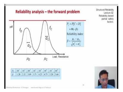
So, this would be comparing C and D side by side and the failure probability is P C less than D and we see the 2 density functions of C and D side by side. D is obviously to the left of C because we want the failure probability to be low enough. What I have marked here on the 2 density functions is the mean of D and the mean of C respectively and the standard deviation of D and the standard deviation of C, just to show the relative scatter the spread in the 2 distributions.
