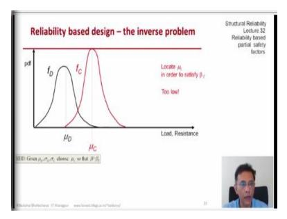
And this is the statement of the inverse problem. We have been given a load, so I have not changed the distribution of the load; it is unchanged from the previous slide. But now the distribution of C is missing, because that is what we need to find out. And so the reliability based design inverse problem is given mu D, sigma D and sigma C, choose the unknown mean of C. So, that beta equals beta target.
