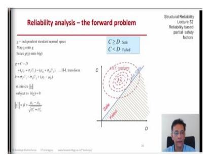
And we have the independent standard normal space u, so we map the basic variables onto this space of u. And hence the limit state function g onto h, so the new limit state is g = 0 becomes h = 0. And let us say we employ the simple second moment transformation or the Hassle-free for transformation, so g = C - D becomes a linear function in h. So, C is mu of C + sigma C times U 1, U 1 being the standard normal random variable and D is mu D + sigma D times U 2.
