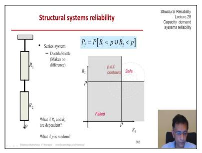
Let us look at the simplest possible configuration of a serious system a two unit system here we have a mechanical system two bars or two springs with strength R 1 and R 2 respectively loaded by an actual load p. So, clearly each of them is loaded by the same load p. R 1 and R 2 are random variables and now there would be a question what is the material behaviour are these ductile are these brittle or are they somewhere in between.
