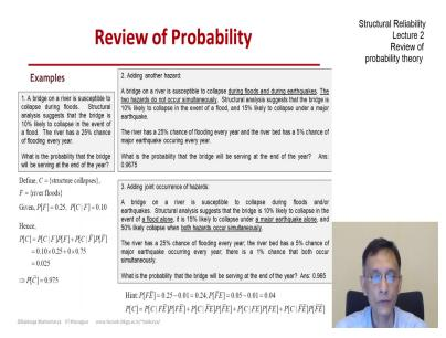
The next example is a structure subject to first one natural hazard and then we will add one more. So, let us read the problem the bridge is 10% likely to collapse in the event of a flood and the river has a 25% of flooding during the year. So, let us define the events carefully there are 2 basic events here C the structure collapses and F the river floods the information given for the 2 probabilities is P of F is 0.25 and P of C given F is 0.1.
