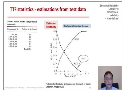
The next example we take up is also from Schumann's book we have here failure data presented in intervals of time. So as you see on the table on the left there were 59 failures between 0 to 1000 hours of test time and then for subsequent thousand hour intervals all the way up to six thousand. So, we have 6 intervals and a total number of 172 items tested. So, the first task will be to estimate the CDF of this item.
