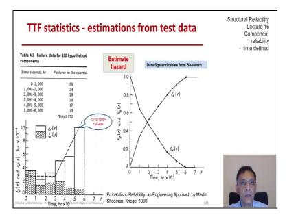
The next task is to estimate the PDF of the time to failure of this component from the same data that is in our table. So, for that let us reproduce the graph from Schumann's book and this particular graph includes both the PDF and the hazard function and according to the author's nomenclature z d stands for the hazard function and f t small f t stands for the density function. So, let us now make sure that we are able to reproduce the PDF values from this data set.
