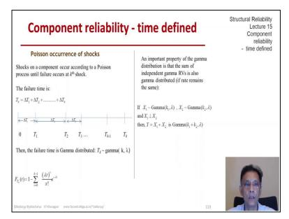
Now continuing the gamma distribution is closed under addition the gamma family provided the rate does not change. So, if we continue adding gammas from the same underlying process defined by lambda gamma k 1 lambda and gamma k 2 lambda if they are independent then their sum would be a new gamma random variable with parameter k 1 + k 2 and the same lambda as before. So, now let us solve one or two examples with this sort of arrival on the time axis.
