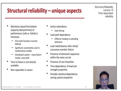
So, first of all our formulations are almost always mechanics based which is known as capacity demand or capacity demand time type formulation uh. So, that is what we call a limit state limitator for performance there could be uncertainties in the mathematical models the systems are distributed in nature and there could be there are generally more than one failure modes many degrees of freedom to describe my system.
