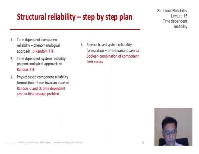
First we are going to look at starting with today's lecture time dependent reliability from a completely phenomenological approach for a component. So, our focus will be the random TTF time to failure. Then the next step would be time dependent system reliability continuing with the TTF approach. So, from element we move to system the third step would be the physics-based component reliability formulation.
