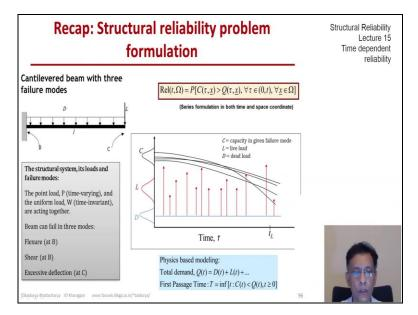
This made things a little more interesting that this example that we looked at it is quite instructive that we have a structure with more than one failure mode. So, in effect this has three elements one of flexure one of shear and one of excessive deflection. That is all fine but things become more interesting when we bring in or when we have to bring in some time dependence in one or more aspects of this problem.
