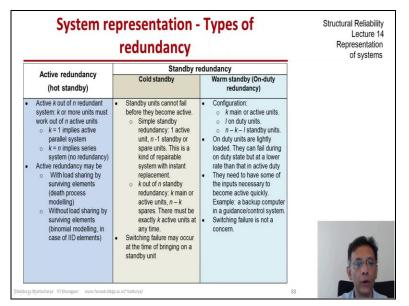
So, but now let us look at the different times of the different types of redundancy that are normally defined in reliability textbooks and look at the different types. So, we broadly have two kinds of redundancy standby redundancy and active redundancy. So, let us first define active redundancy. An active redundancy is basically all elements are loaded to the full extent and there could be in general it is k out of n redundancy.
