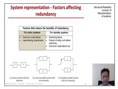
So, now we have discussed this just now but let us try to put things together that how is redundancy you know not as much as it might seem at first glance. So, factors that reduce the benefit of redundancy or additional members for active systems it could be common mode failure it could be load sharing or for standby systems it could be due to switching failure or even failure of standby units before they come online and some amount of common mode failure also.
