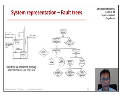
The next example converts a similar water related problem flooding in a in a basement sump pump system and we will just look at this diagram it is a nice diagram taken from hang and tang look volume two and it is possible to convert this into a fault tree. So we have the top event flooding in basement that can happen either if the pump system fails or the inflow exceeds the pump capacity and then that second event requires no further development.
