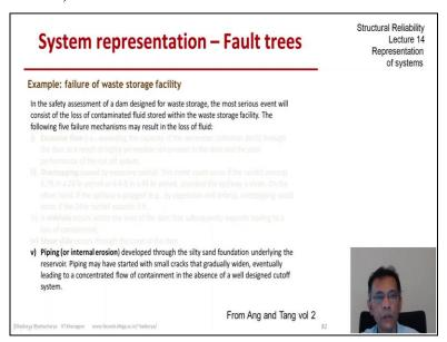
In the next three slides let us take a look at how to convert a set of high level engineering statements about the performance of a system can be converted into the corresponding fault tree for the system. So, the first example is a toxic wastewater storage facility. And let us look at the failure modes one by one. These are a bit wordy. So, if you would like to pause the video and take your time readings please do so.
