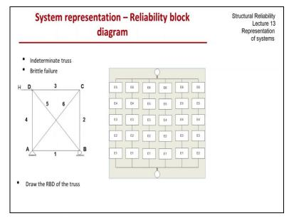
So, the structure has failed. So, if we do this again and again for various combinations pairwise for lost elements we will see that this any 5 have to work any five of these six elements have to work. So, we could draw an RBD and say that you know there are six elements E1 through E6 and five out of six configuration which when expanded looks like this there are 6 ways of choosing five elements from the group of six.
