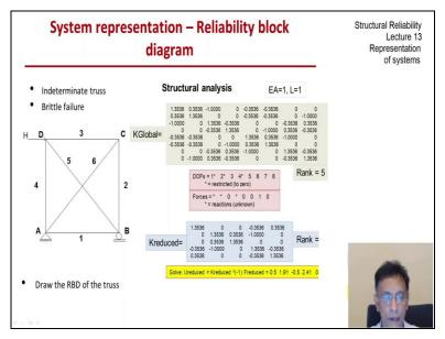
So, this is the truss that we would like to analyze this has 6 elements two diagonals elements five and six simply supported at A and B, A is a hinged support and B is a roller support uh. So, we need to draw the RBD of the truss again depending on our understanding of the structure and how its boundary conditions are what its material is and. So, on we can find its reliability block diagram by inspection or we might have to do some structural analysis as well.
