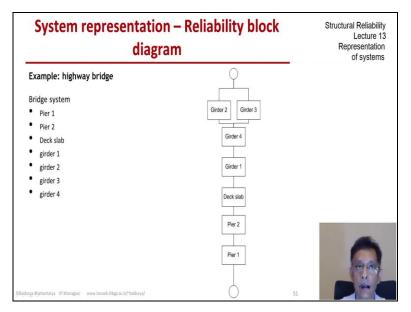
This is a little more complicated than this 7 member determinant truss. We if you remember we had a bridge system that involved two peers 1 deck slab and 4 girders and the logic that we agreed upon for the bridge was that each of the peers is essential for the functioning of the bridge as is the deck slab. But for the girders the end girders on either end girder one and girder four are essential but if two fails or three fails separately then the bridge is still okay.
