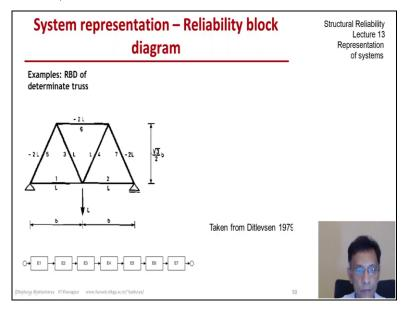
Let us start with a very simple example this is a determinate truss taken from Ditleven's 1979 book since this is a determinant truss any element failing is tantamount to system failure. So, the system is in effect a series system and the reliability block diagram for this system would be just the 7 elements of the 7 truss elements connected in series. So, as I said this RBD that you see at the bottom of the page it does not in any way mean that that's how the elements are connected.
