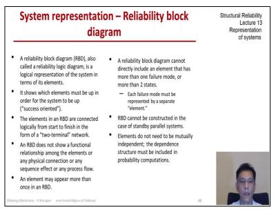
And RBD also called a reliability logic diagram is a logical description of the system in terms of its elements and we have seen some examples obviously in the last few weeks. It shows which elements must be up in order for the system to be up. So, it is a success oriented approach the elements in a RBD are connected logically from start to finish. So, we have a start terminal and an end terminal.
