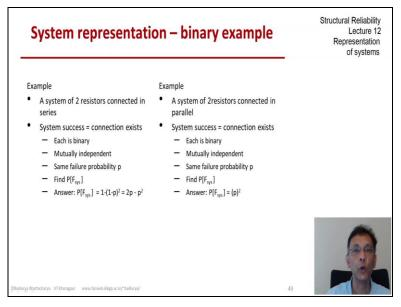
Let us solve some problems involving a system composed of just two elements. The simplest we have already looked at in various situations and one example is here on the screen that a system consists of two binary units, two resistors connected in series and the system success is defined as connection exists across these two each of these resistors is binary in nature they are mutually independent.
